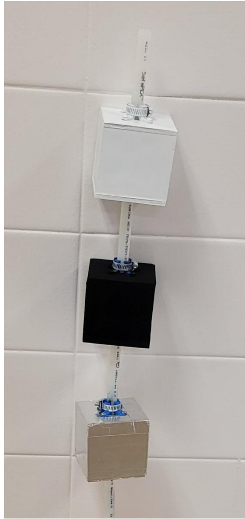
Figure 2: The silver, black and white boxes as part of the color box experiment with the polyethylene tube threaded through.
