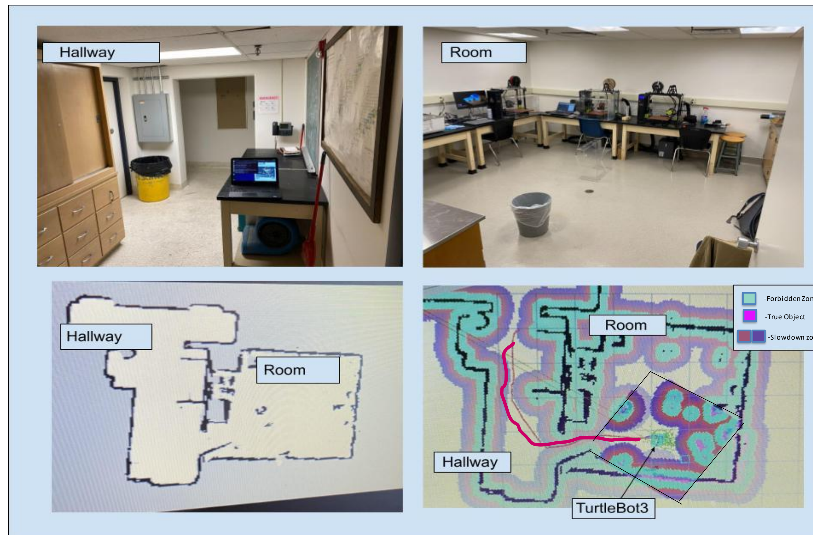
Figure 2: The top two figures show the actual environments that the LDS-02 scanned. The bottom left shows the baseline map of the room generated using the ROS2 Cartographer. The bottom right shows the map file combined with the LiDAR data (the square seen around the TurtleBot3) that are used to navigate to a desired target location. The red line is the TurtleBot3's path to the target.
