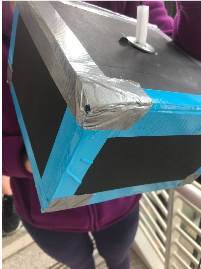
Figure 13: Damage from Stair Test
