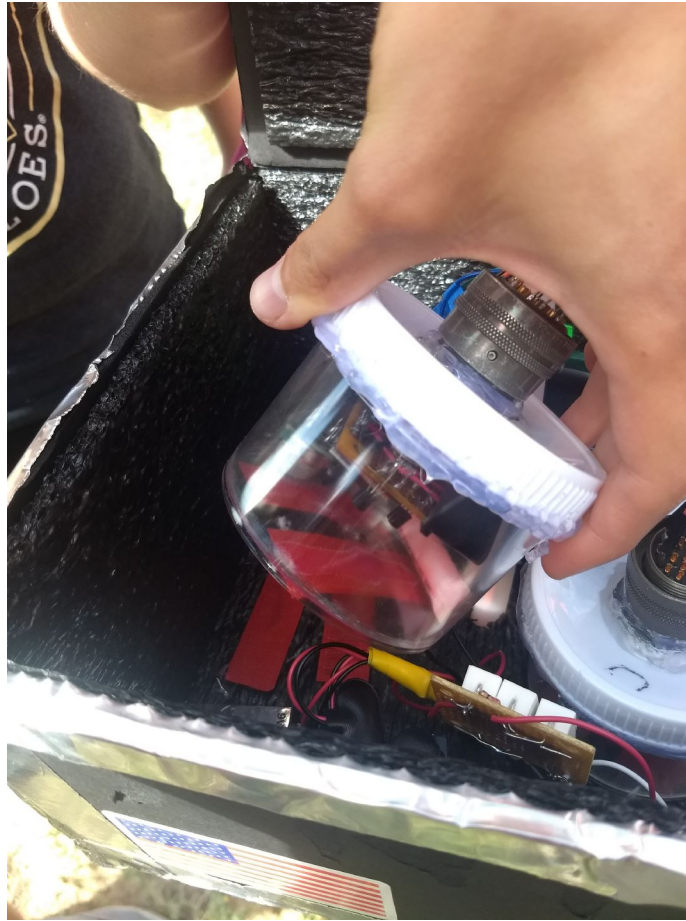
Figure 18: Final method of sealing the jar
