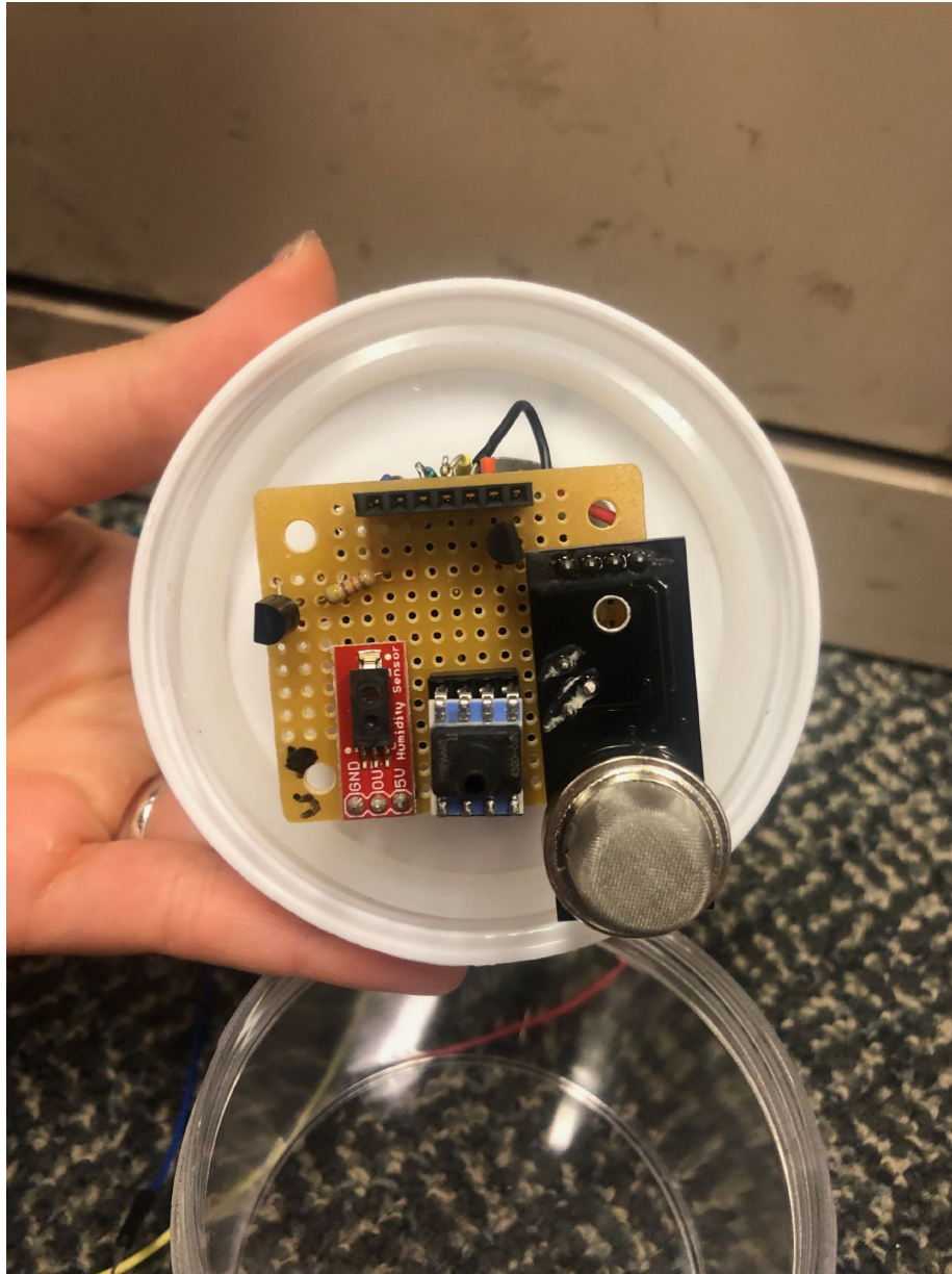
Figure 7: Sensors included within Polystyrene Jars
