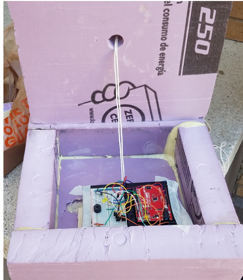
Figure 9: Dummy electronics placed in outer shell for swing test.
