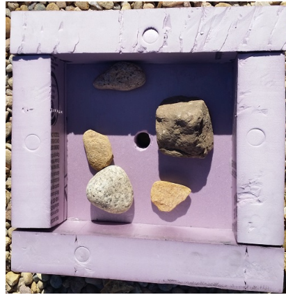
Figure 7: Dummy load placed in outer shell for drop test.
