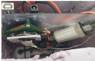
Figure 6.6 – Frost on the board
