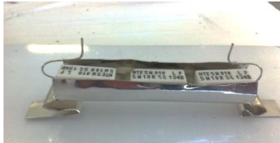
Figure 3.16: Heater unit before being placed inside of PVC Piping
