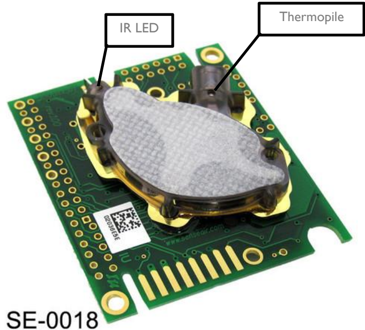
Figure 3.6: K-30 CO_2 sensor. (co2meter.com)
