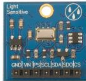
Figure 3.12: Altimeter Sensor Source: www.parallax.com
