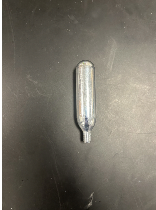
Fig 4.2.1: The CO2 cartridge we planned to use for the test chamber. Photo by Colin Borror
