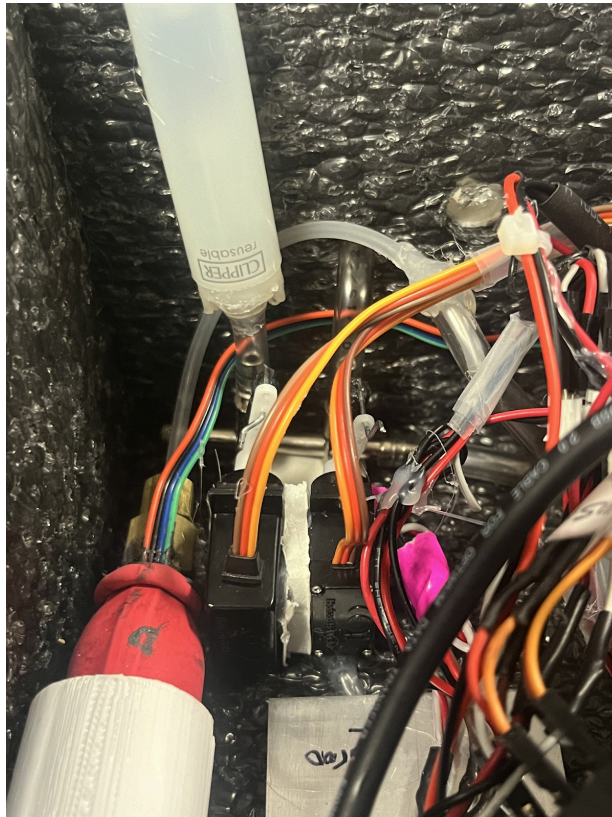
Fig 4.2.2: The top of the test chamber, lighter, and servo/valve manifold after assembly. Photo by Marco Villasuso
