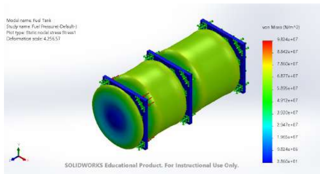
Figure 13: FEA: Main Fuel Tank von Mises Stress
