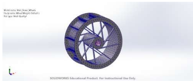
Figure 15: FEA: Wheel Mesh
