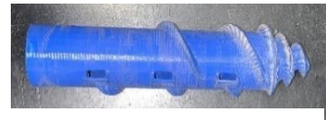
Figure 23 Moe - eighth and final drill iteration; used in drilling mechanism.
