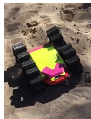
Figure 30: TAD V1 with updated "Beluga" wheels.
