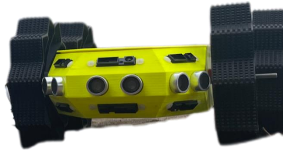
Figure 25: TAD V1 with TPU wheels.
