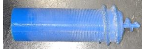
Figure 19: Fives - fifth drill iteration - second auger design.
