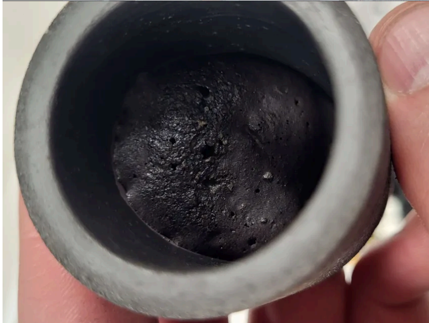
Figure 9. The LRS in the crucible from the induction sintering experiment appears to be black and glossy. This implies that it went past solid state sintering and became molten.
