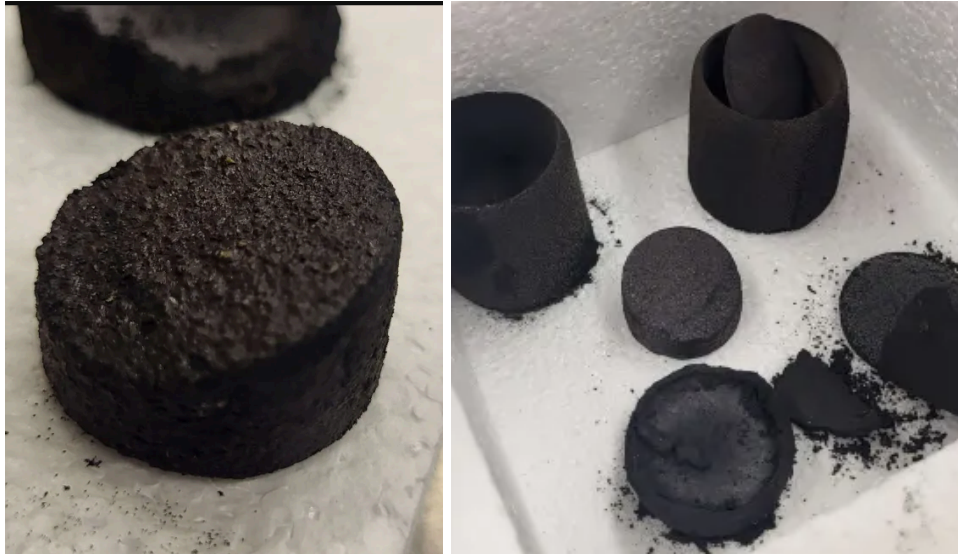
Figure 3 & 4. A fully sintered puck of LRS can be seen on the left. The picture on the right shows the crucibles after the kiln sintering experiment.
