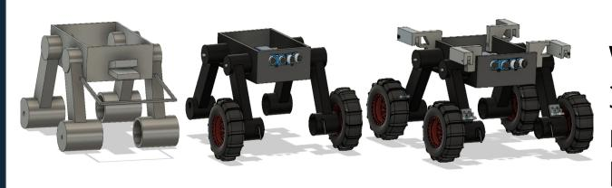
We started with computer aided 3D design trying to develop a model we could then print and build off of.
