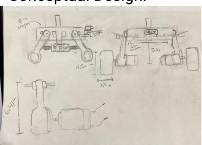
Most important features of our robot from the start: Lift from the ground Main housing unit 4 legs housing motors Wide base Front sensor
