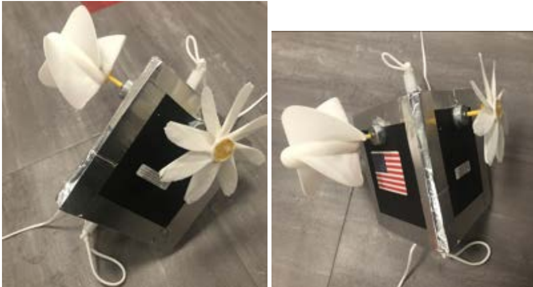
Payload Exterior with two PLA printed turbines
