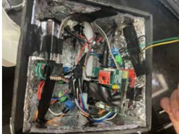
Interior of Final Payload Powered by 5V Battery
