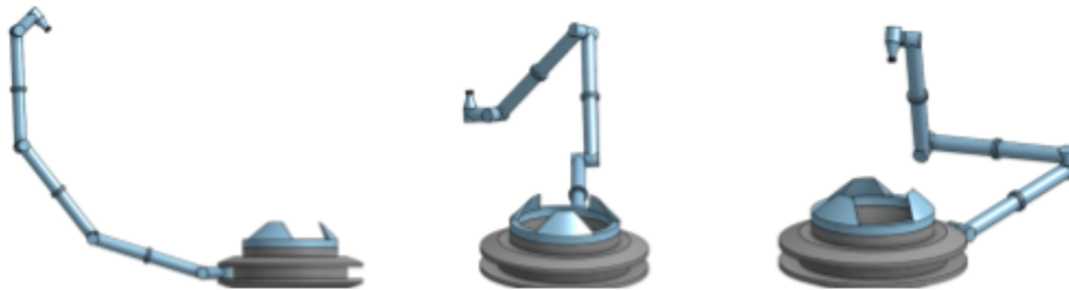
Figure 8: Three possible camera angles for up close and farther away views of the docking area
