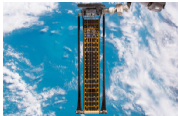
Figure 10: Fully extended ROSA on the ISS (Redwire Space, 2022)
