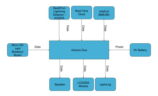
Figure 1: PLLAWDA Block Diagram
