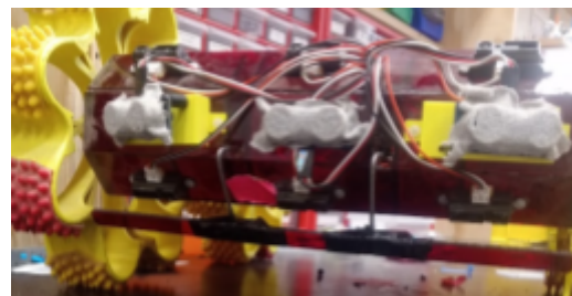
Figure 6: 6 Infrared Sensors for navigation both rightside up and upside down.
