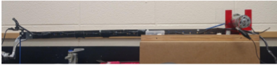
Figure 11: Retrieval arm with drill motor.
