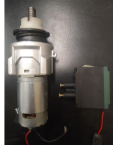
Figure 4: Drill motor vs Vex motor
