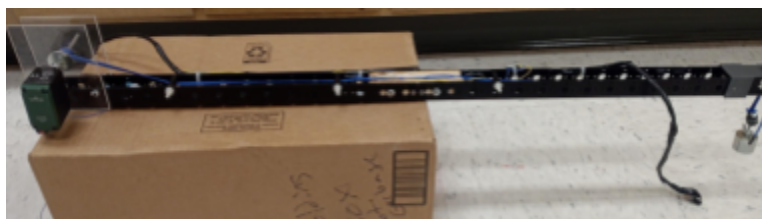
Figure 12: Updated retrieval arm with Vex Motor
