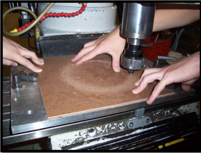
Template for foam core cut on CNC
