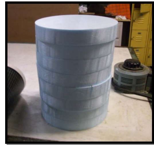
Stack of foam core sections (pre-hollowed)
