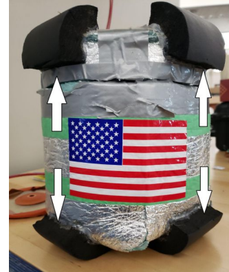
Fig. 5.14: The white arrows point to the force dampener upgrades
