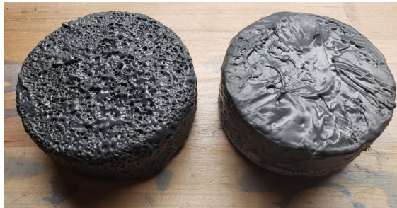
Fig. 5.17: Test 1- vacuumed JB Weld (left) and Test 2- regular cured JB Weld (right)
