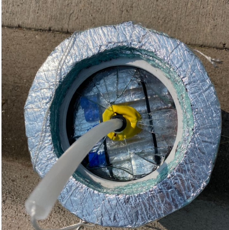
Fig. 5.13: Radial glass shatter in the first drop test
