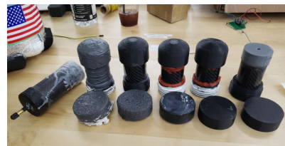
Fig. 5.15: From left to right; Bike Pump test, JB Weld full coating, Potted JB Weld, Rubber inner lining, PVC inner lining and control
