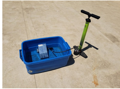
Fig. 5.16: Bike pump test setup.
