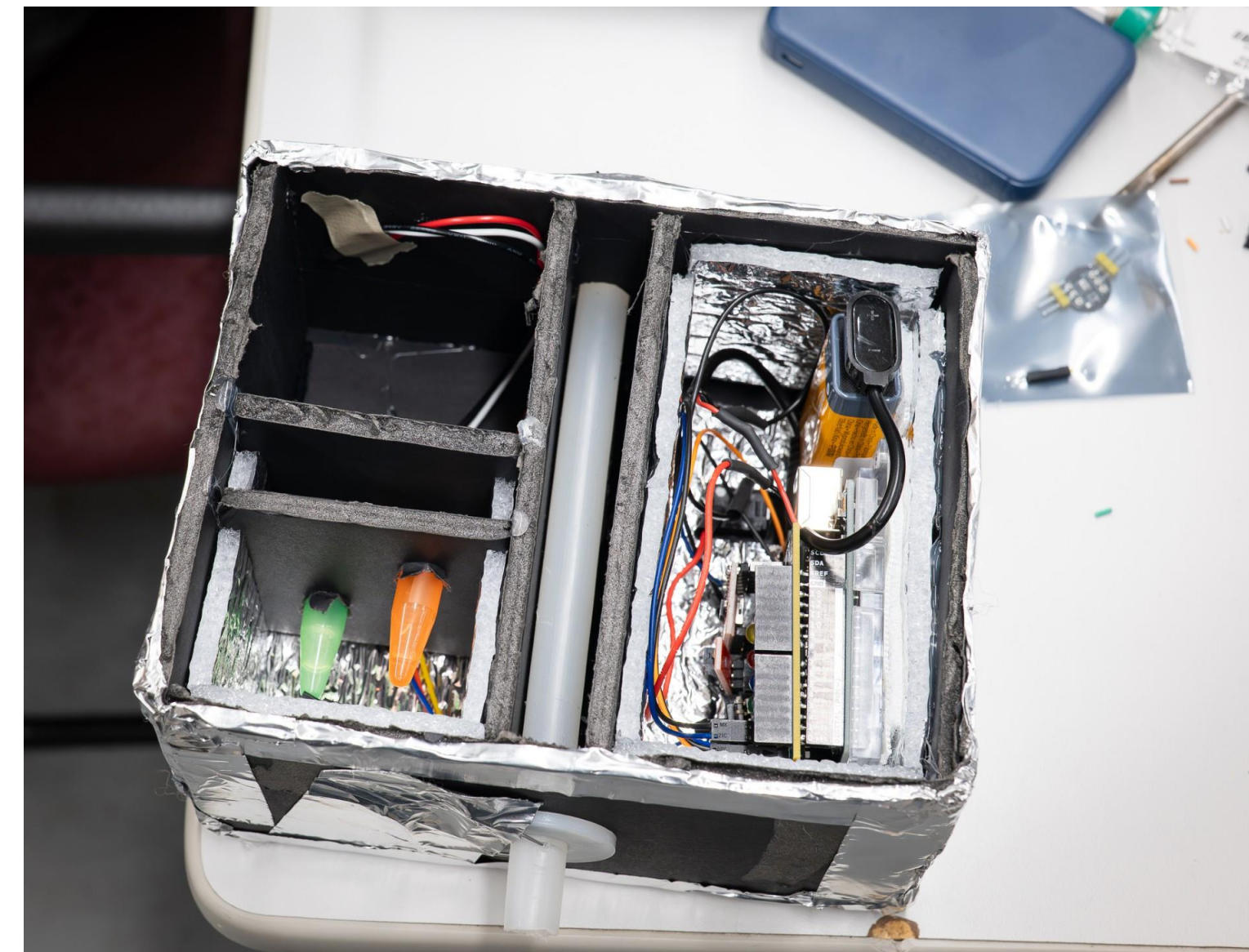
Fig 2: Payload layout with data collection system (right) and worm storage area (left).
