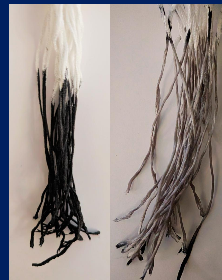
Figure 7. Thermochromic pigments shown before and after temperatures reach 85 F
