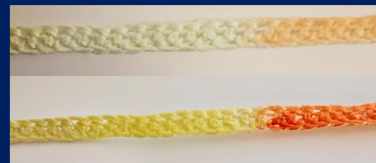
Figure 6. UV Reactive Pigment shown before and after exposure to sunlight
