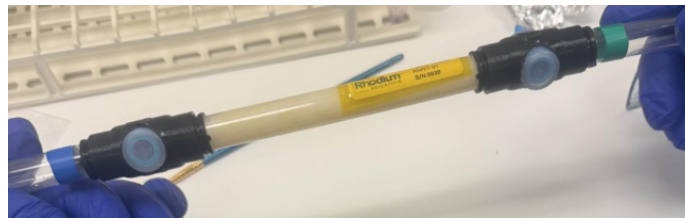
Figure 3: Capillary transport visualisation: a prototype RhFET tube was filled with dyed deionised water to test capillary flow through the cotton wick. The coloured liquid migrated evenly along the wick and into the biological chamber without leaks, confirming that passive hydration can saturate the seeds uniformly in a diffusion-dominated environment.
