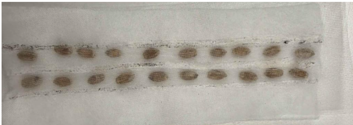
Figure 4: Seed-pocket arrangement trial: seeds were placed between a cotton wicking strip and an overlaid nylon mesh sewn into pockets to keep them evenly spaced. This configuration prevented movement during handling and ensured the wicking pathway remained clear for capillary flow. The trial confirmed that the seeds stay in place and do not block the valves.
