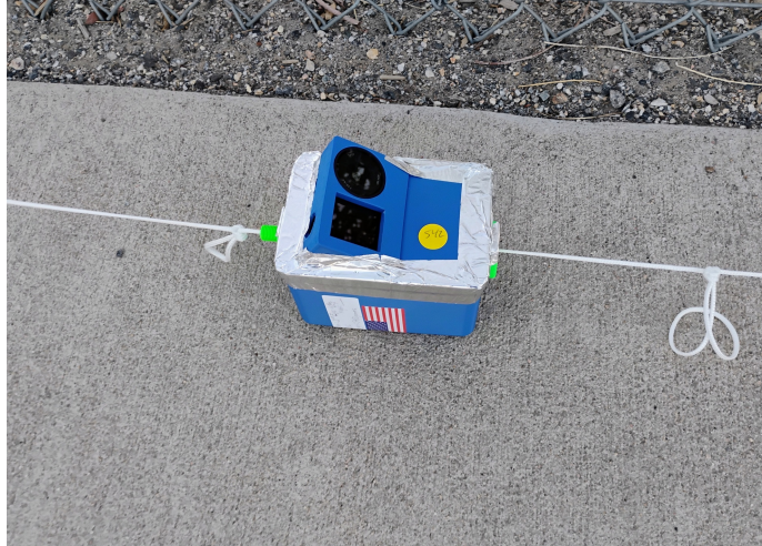
Figure 4: Redesigned payload strung on flight string prior to payload launch
