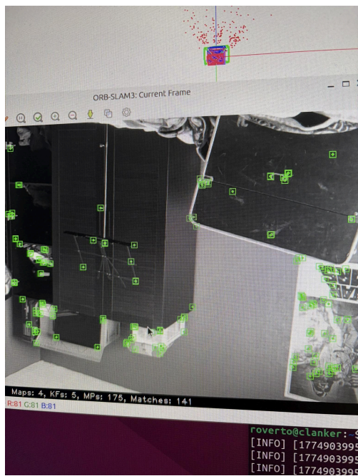
Figure 2: An image of the SLAM detecting ORB points on a camera frame.
