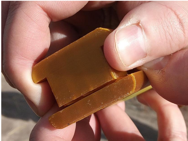
Figure. 3: Example of layer separation failure
