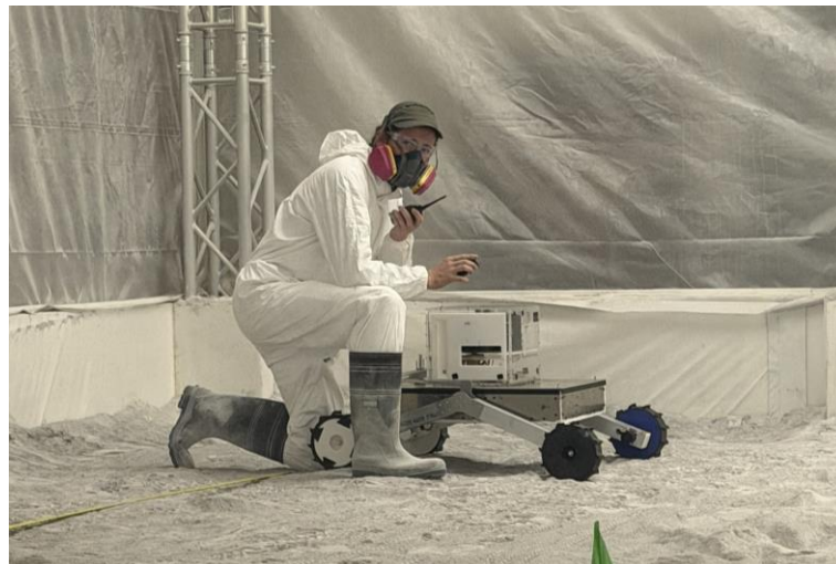
Figure 1: Systems Engineer, Jonathan Leites, with integrated Rover-HDM system inside Mines Lunar Regolith Test Bed (Source: Observer, February 2026).
