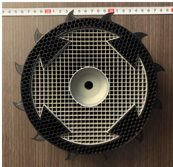
Figure 3: Unfinished 3D-printed wheel prototypes showing internal structure and overall design. A ruler in the background (centimeters) provides scale. (Source: Robotics Team, April 2026)
