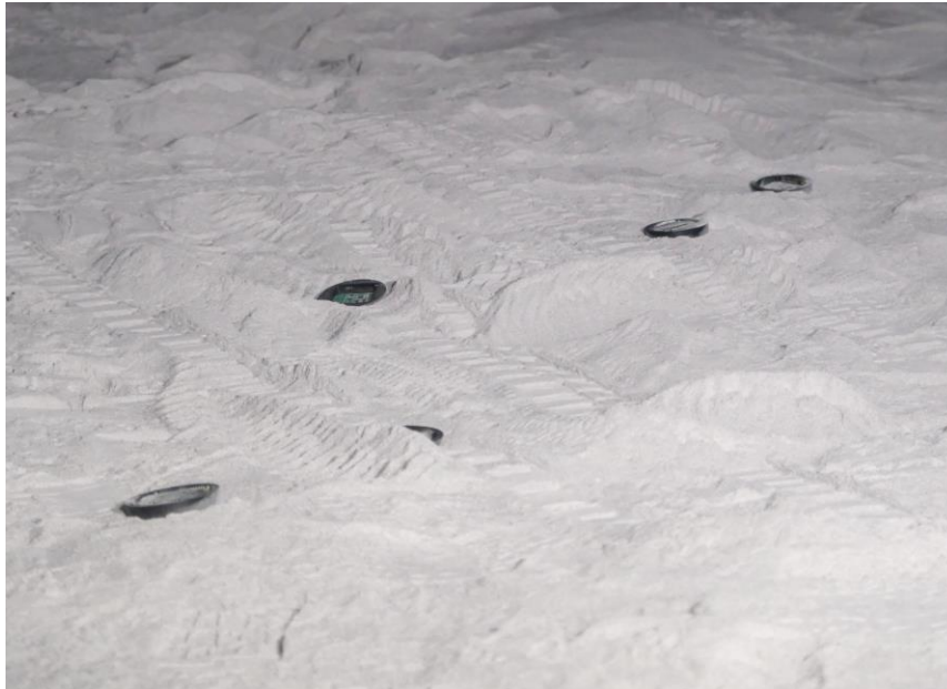
Figure 6: LunaSat V7 Pucks after landing in regolith at the Colorado School of Mines Test Bed (Source: Team member photographer)
