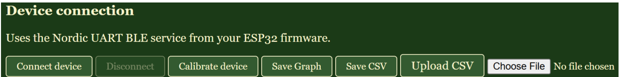
Figure 6: BLE connection buttons, data attaining buttons, and angle calibration button.
