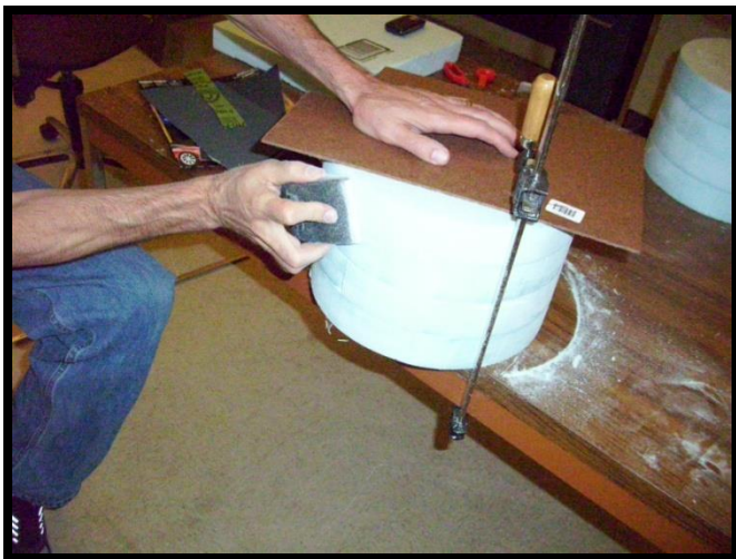
Sanding of foam core sections
