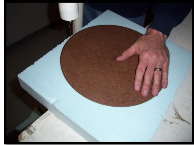
Cutting of foam core section with hot wire cutter
