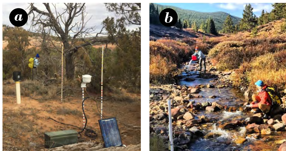
Figure 31: Examples of low-cost headwater catchment monitoring. (a) Cameras pointed at demarcated poles measure snow depth; (b) pressure transducers within PVC pipe track water depth in streams. Salt dilution stream discharge measurements are being conducted in (b).
