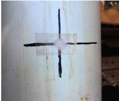
Place scotch tape over the sanded region, place marks on tape for precision placement.
