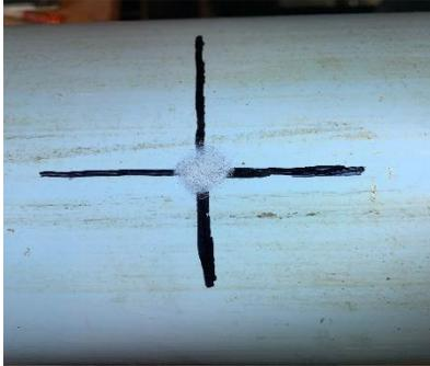
Use both fine and course sand paper to sand the section of pipe the strain gauge will sit on. Sand in several directions for better adhesion.
