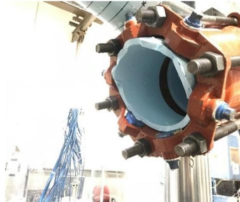
(b) Post-test showing pipe fracture
