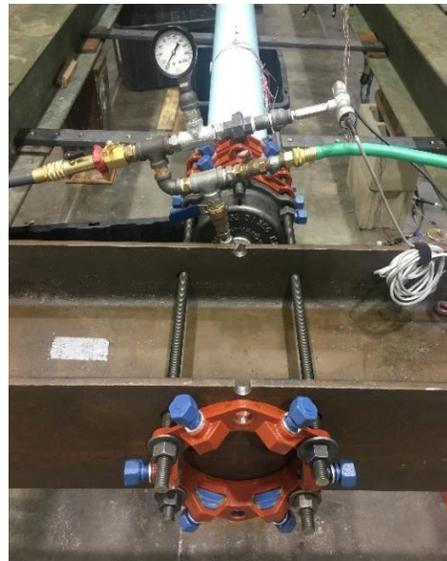
Figure 2.7. Fixed end (west) with water intake and pressure valve
