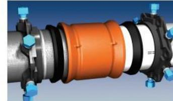
3. Center the sleeve body over the ends of the pipes while maintaining a 1/2" to 1" gap between the pipe ends. Slide the gaskets and end rings toward the sleeve body.
