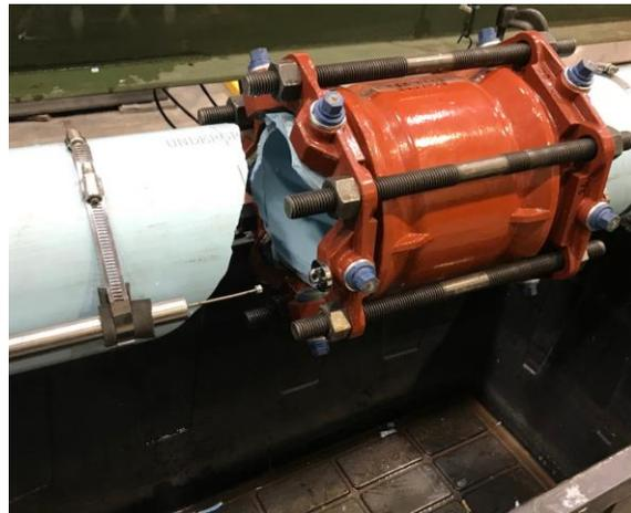
Figure 3.19. Failure at west joint for PT08
