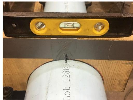
Figure 2.4. Identifying the pipe coordinates (crown, invert, and spring lines)
