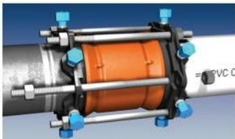
4. Install the threaded rods and hand tighten the nuts on each end. Gradually tighten the nuts in an alternating manner until the proper torque value has been reached, while maintaining the same distance between the rings and the ends of the body at all points around the rings. For 4 inch through 24 inch torque to 75 - 90 ft.-lbs., for 30 inch and greater torque to 120 - 150 ft.-lbs.
