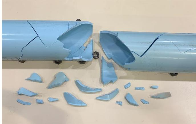
Figure 3.26. Failure at joint for PT14
