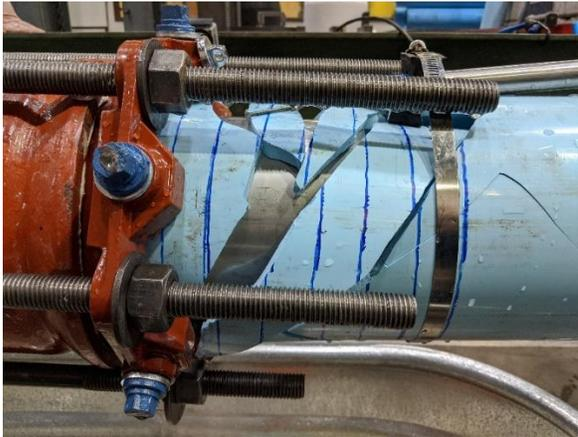
(a) Fracture of the pipe
