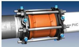
5. Hand tighten the actuating screws until all wedges are touching the pipes. Continue tightening the screws in an alternating manner until the torque limiting heads twist off. The screws may bottom out during this step.
