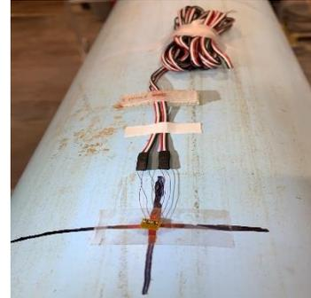
Open Strain Gauge package, tape wiring onto pipe so that the gauge is easy to work with. Place the gauge onto the tape, lining it up with the marks as close as possible.
