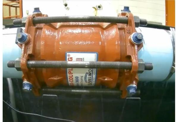
(b) Initial Slipping, No Leak
