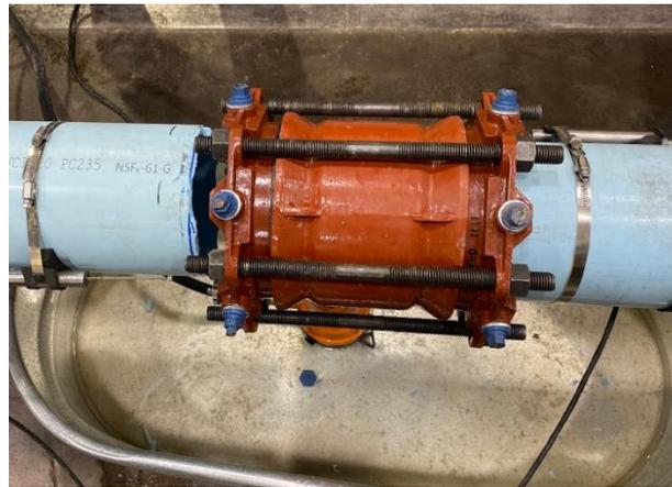
Figure 3.33. Failure at coupling for PT15
