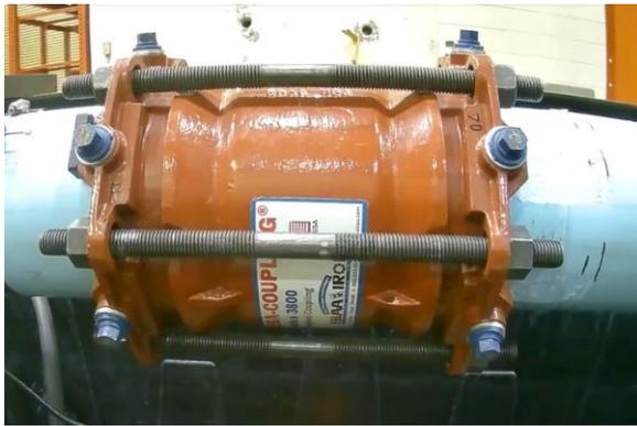
(c) Final Slipping Position Without Leak
