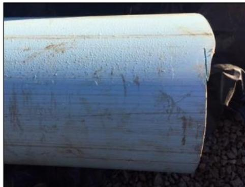
Figure 7.3. When stress is not relieved in the pipe during the cutting process, the forces in the pipe may cause the cut to be uneven.
