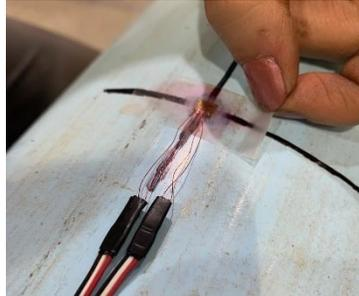
Remove tape slowly, making sure the gauge is bonded to the pipe. If the gauge lifts from the pipe, continue to press onto the gauge for an additional two minutes.
