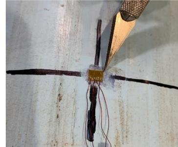
Use a knife to attempt to lift the corners of the gauge from the pipe. If any part of the gauge is not bonded to the pipe, remove the gauge, and repeat the process.
