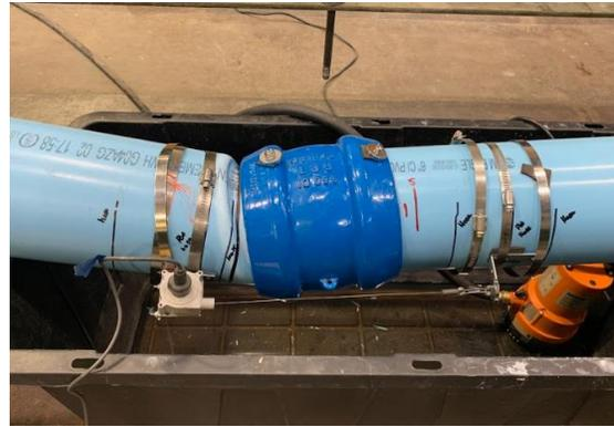
Figure 4.7. Buckle at east joint for PC06
