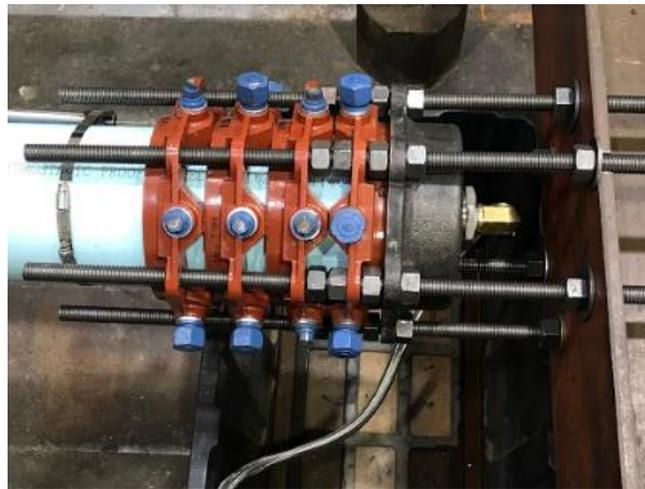
Figure 4.2. Megalug end restraint orientation for compression
