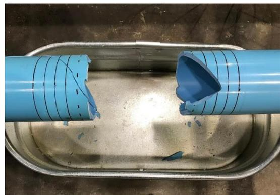
Figure 5.6. Failure at joint for PS12
