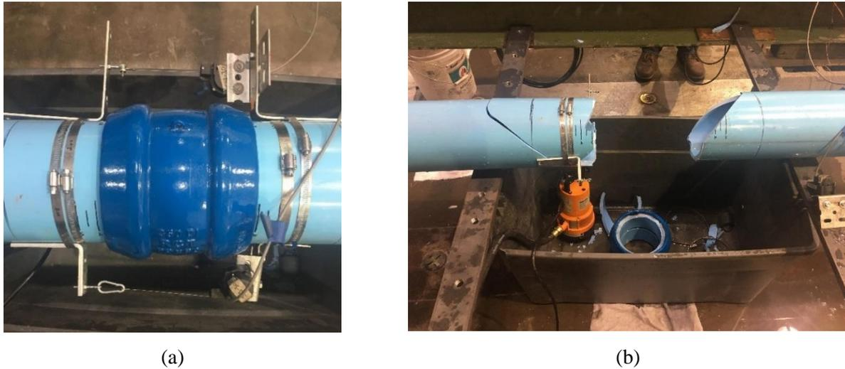
Figure 3.5. Specimen PT02 (a) before and (b) after axial tension test
