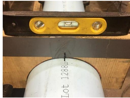
Figure 2.4. Identifying the pipe coordinates (crown, invert, springlines)
