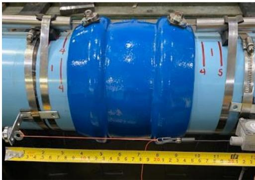
Figure 3.13. LVDTs (top) and string potentiometer (bottom) locations for PT05
