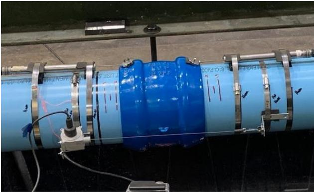
Figure 4.6. LVDT and String Potentiometer locations for PC06
