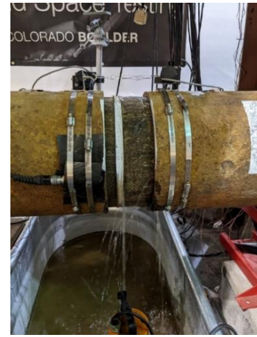
Figure 56. The gap opening in the failed specimen for C01
