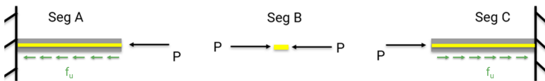
Figure 3. Fully bonded approach schematic with friction from pipe-soil interaction
