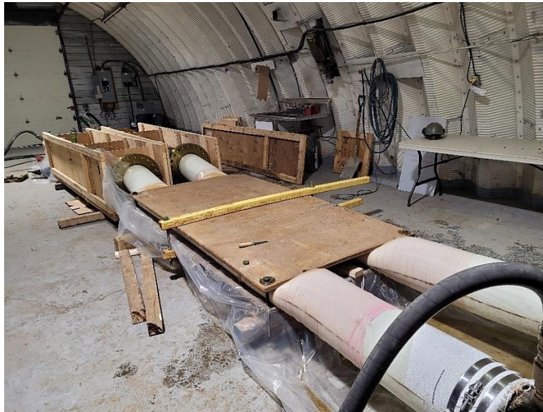
Figure 5. Preparation of AQUA-PIPE™ specimens, including full-scale specimens (rear) and plates for material testing (center, covered by plywood)
