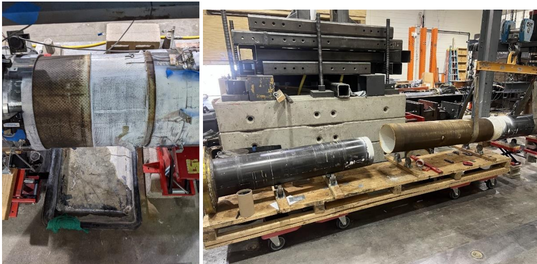
Figure 75. Image of (a) gap opening after S02 pull to failure and (b) removal of liner from host pipe after test
