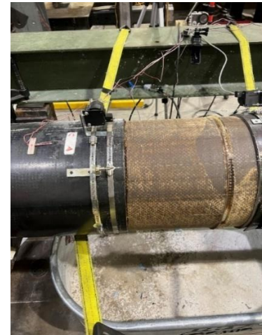
Figure 40. Gap opening in the failed specimen S01
