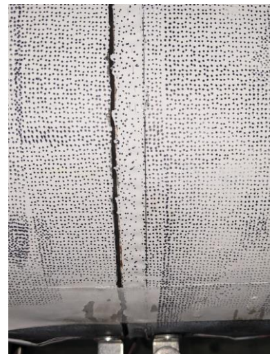
Figure 84. S03 gap after the parallel excavation bend test near the invert (north side of specimen)
