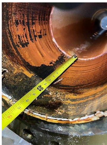
Figure 96. Specimen S03, after all ultimate axial test cycles(including post pull friction cycles) had been applied to the specimen, showing East side fully debonded
