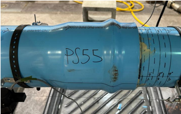
Figure 4.43. PS55 joint before testing
