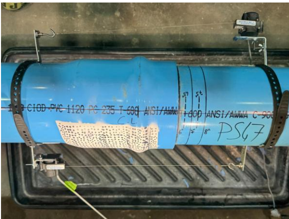
Figure 4.6. PS47 joint before testing
