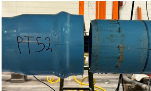
Figure 3.40. After failure for PT52
