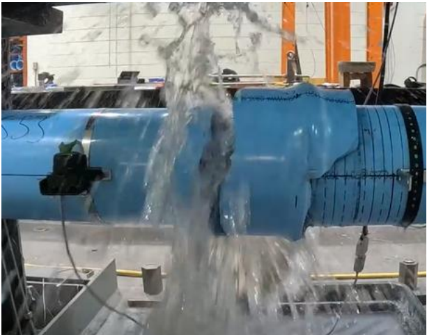
Figure 4.27. PS53 failure moment (The close-up view of North side)
