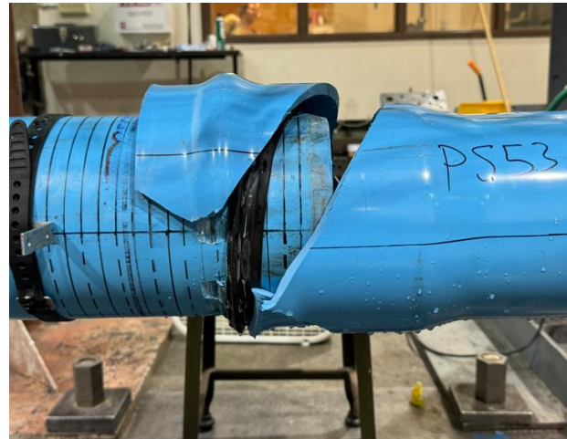
Figure 4.28. PS53 fracture at the bell side of the joint (The close-up view of South side)
