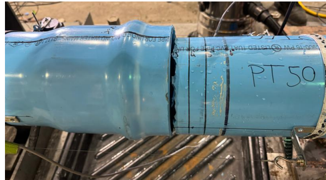
Figure 3.26. Fracture at the spigot for PT50
