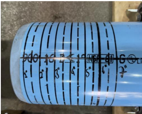
Figure 2.5. Marked measurements on spigot
