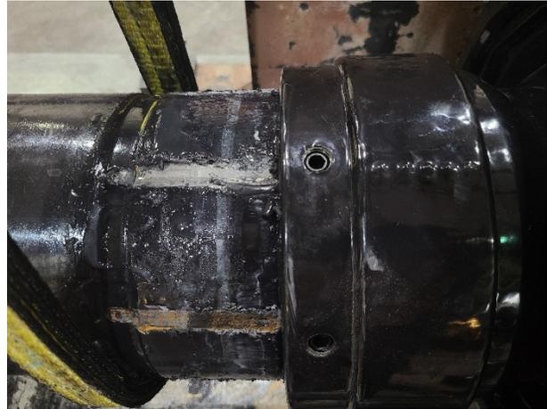
Figure 4.11. Bolt shearing after completely pulling out joint
