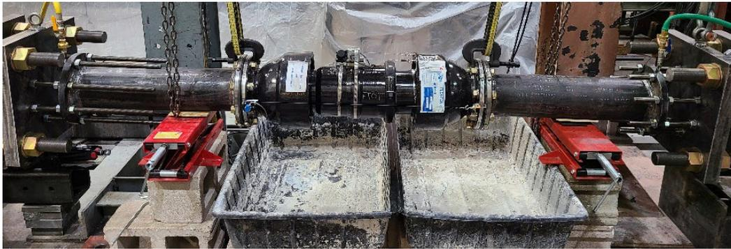
Figure 2.2. FEJ specimen in test frame
