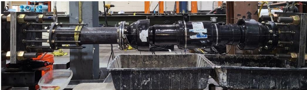
Figure 2.3. FBFEJ specimen in test frame
