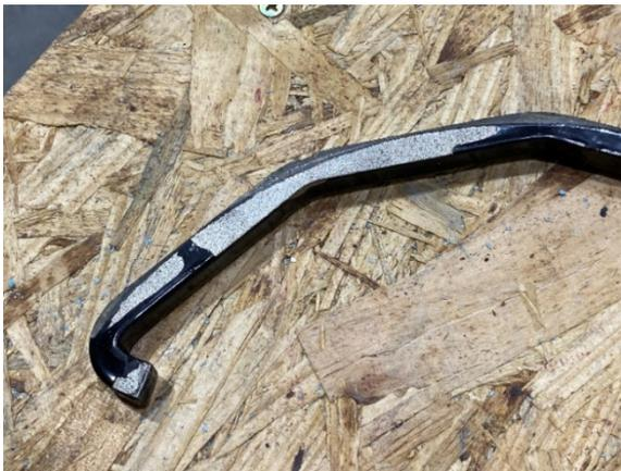
Figure 4.3. Shearing on West retainer ring
