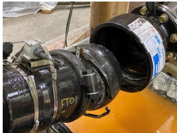
Figure 4.2. FEJ failure at West bell
