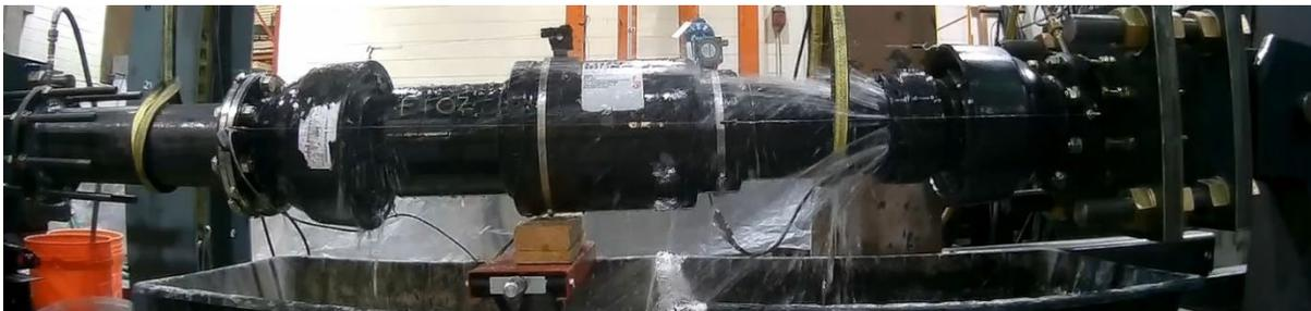
c) Final joint failure at West end
