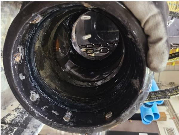
Figure 4.12. Bolt shearing inside West bell
