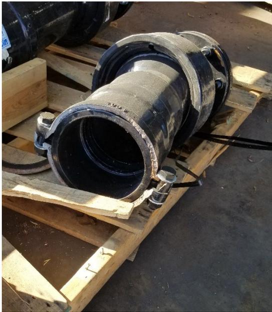
Figure 4.19. Pressure test 406F20 failure at stop collar
