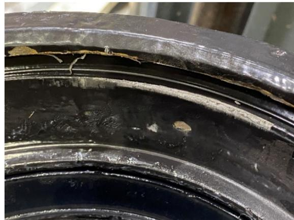
Figure 4.4. Shearing inside West bell
