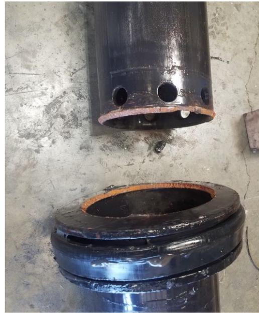
Figure 4.20. Pressure Test 4406F20B failure at telescoping joint
