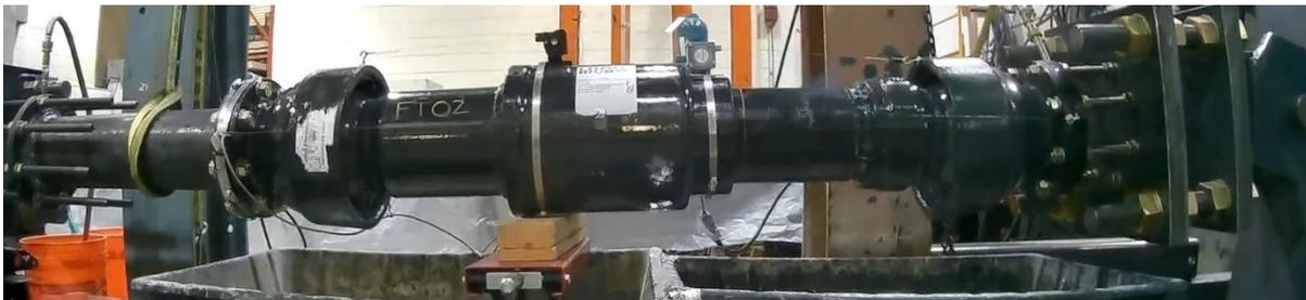
b) Bolt failure when joint was fully extended
