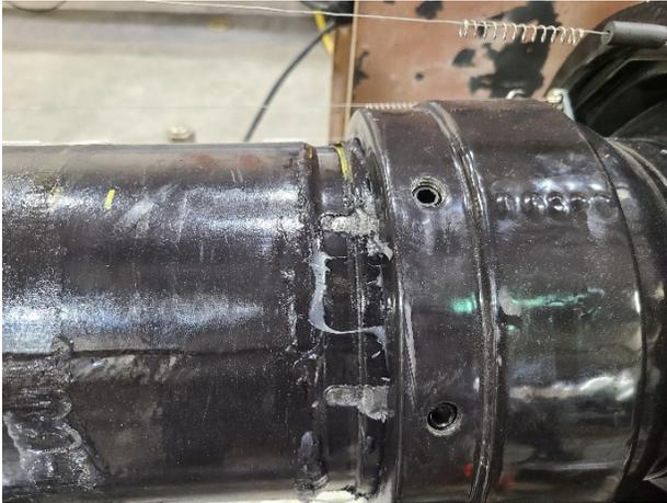
Figure 4.10. Initial FBFEJ failure due to bolt shearing at West end
