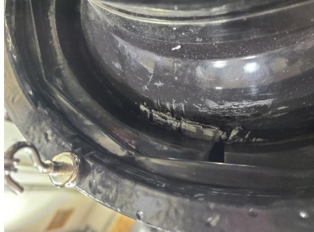
Figure 4.13. Shearing at West ball joint
