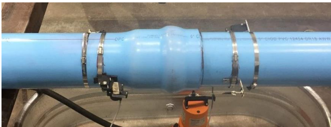
Figure 1.1. Example of a typical bell/spigot joint.
