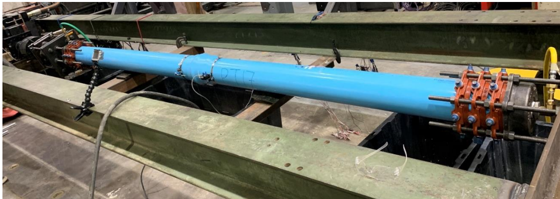
Figure 2.1. Typical setup of pipe assembly in the load frame
