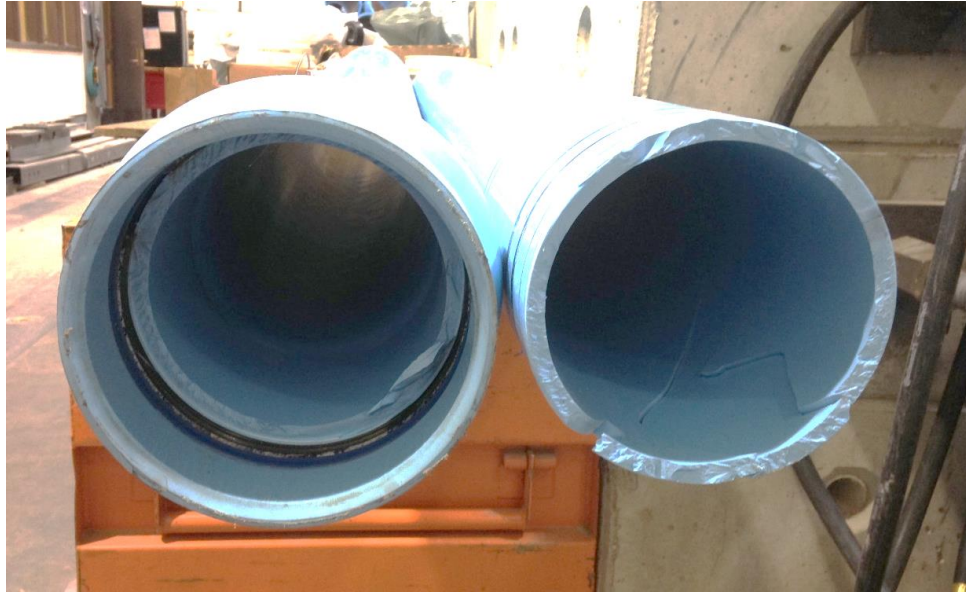
Figure 4.10. PS20 joint failure.
