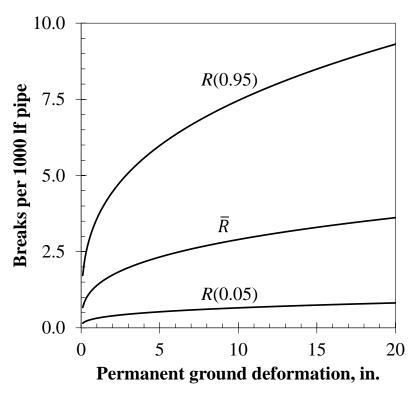
Figure 7. Eidinger (2001) pipe lique faction vulnerability for  $K_2 = 1.0$ , mean and 90% bounds
