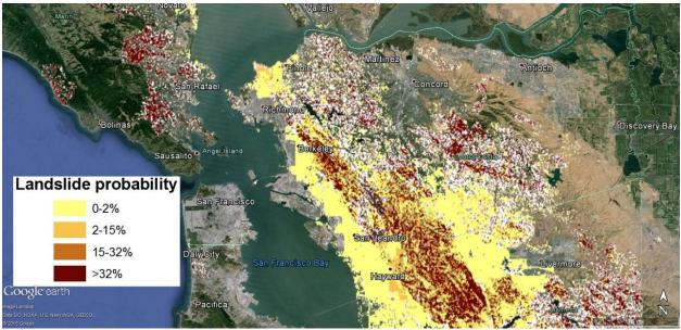
Figure 32. Mainshock landslide probability near EBMUD service area
