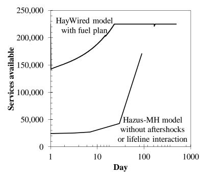
Figure 27. Comparison of the present model with that of Hazus-MH, as applied to SJWC
