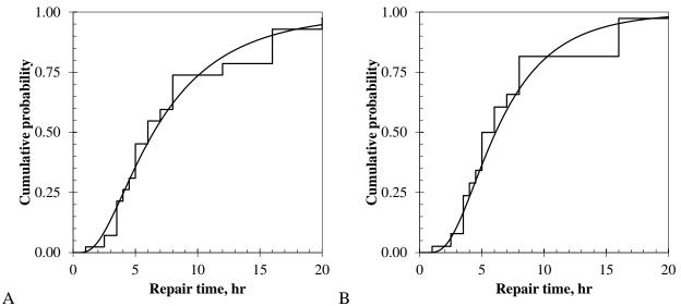
Figure 9. Repair times based on data from Schiff (1988): (A) all repairs (B) excluding repairs to large diameter pipe
