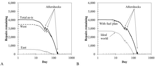
Figure 41. EBMUD repair progress in the Hayward Fault sequence (A) under as-is conditions, showing repair progress east and west of East Bay Hills, and (B) under several conditions, total for the system
