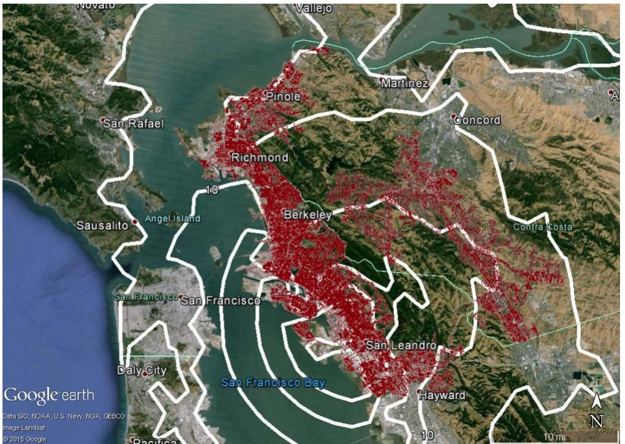
Figure 34. EBMUD water supply system with Oakland M 5.42 aftershock PGV contours
