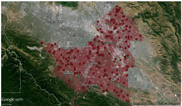
Figure 23. Simulated repairs in SJWC buried pipelines in Cupertino M 6.4 aftershock
