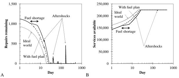
Figure 28. Benefit of replacing AC and CI pipe with ductile iron: A) repairs remaining versus time and B) services available versus time
