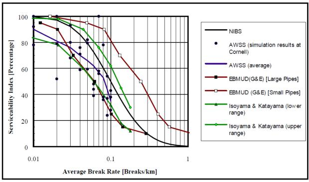
Figure 4. Hazus-MH model of serviceability. Hazus uses the curve labeled "NIBS."
