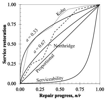
Figure 8. Parametric restoration curves with Kobe and Northridge experience
