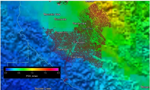
Figure 15. SJWC system map with mainshock peak ground velocity
