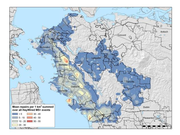
Figure 37. Buried water pipeline damage heatmap for the entire Hayward Fault sequence in EBMUD's service area
