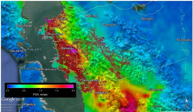
Figure 30. EBMUD water supply system with mainshock peak ground velocities
