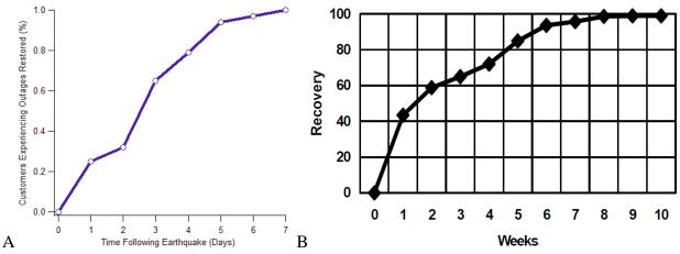
Figure 5. A. Restoration of water service after the 1994 Northridge earthquake and B. After the 1995 Kobe earthquake
