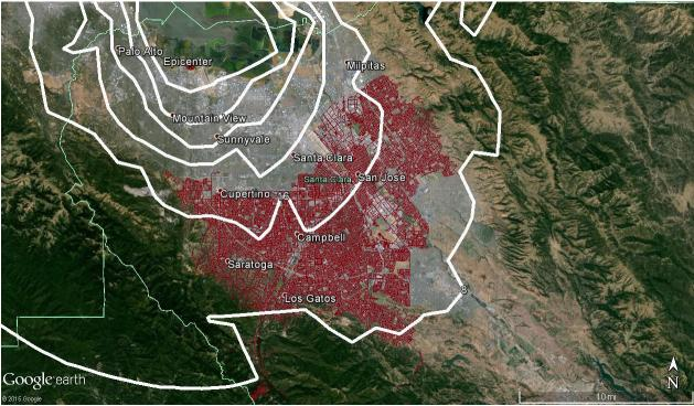
Figure 18. SJWC system map with M 6.4 Mountain View aftershock PGV contours (increments of 0.08 m/sec)
