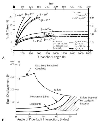
Figure 2. A. Tolerable fault offset vs. unanchor length in continuous pipe (O'Rourke 2003, citing Kennedy et al., 1977), and B. Tolerable fault offset versus pipe-fault intersection angle in segmented pipe (O'Rourke 2003, citing O'Rourke and Trautmann, 1981)
