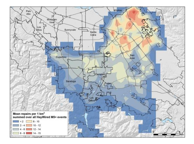
Figure 21. Buried water pipeline damage heatmap for entire the Hayward Fault earthquake sequence in SJWC's service area
