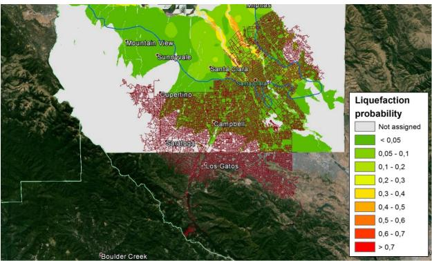
Figure 16. SJWC system map with liquefaction probability
