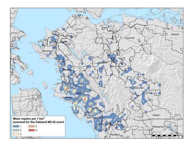
Figure 36. Buried water pipeline damage heatmap for the most-damaging aftershock in EBMUD's service area
