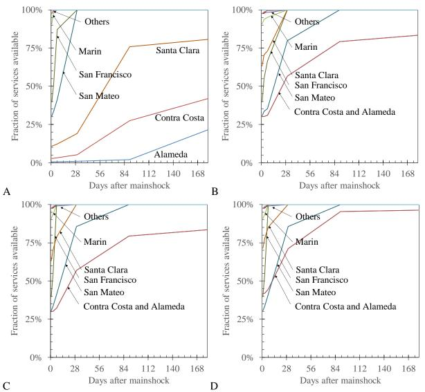
Figure 43. Water restoration (A) according to initial Hazus-MH calculations (B) after adjusting for repair-crew availability and lifeline interaction, (C) after all utilities have implemented a fuel plan, and (D) ideal-world conditions. Curves in B, C, and D use the more-detailed case-study calculations for Contra Costa, Alameda, and Santa Clara counties instead of Hazus-MH.
