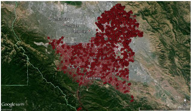
Figure 22. Simulated repairs in SJWC buried pipelines in Hayward Fault mainshock
