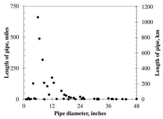
Figure 14. SJWC pipe quantities by diameter
