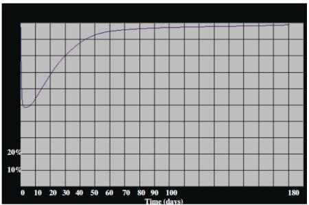
Figure 1. Shake Out water restoration in MMI VIII or higher, where the vertical axis denotes fraction of customers receiving service (Jones et al. 2008)
