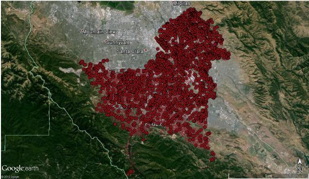
Figure 24. Simulated repairs in SJWC buried pipelines in Hayward Fault sequence
