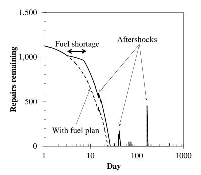
Figure 25. Simulated repair timeline of San Jose Water Company, with and without fuel management plan
