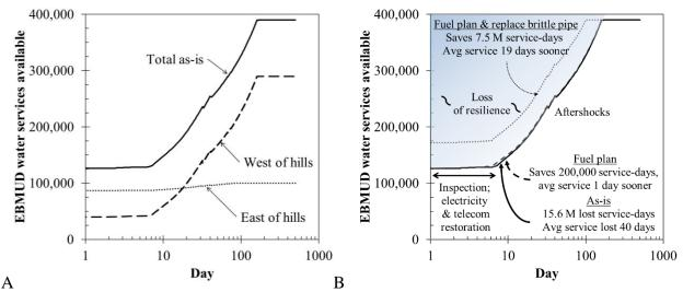
Figure 40. EBMUD restoration curves in the Hayward Fault sequence: (A) under as-is conditions, showing service east and west of East Bay Hills, and (B) under several conditions, total for the system
