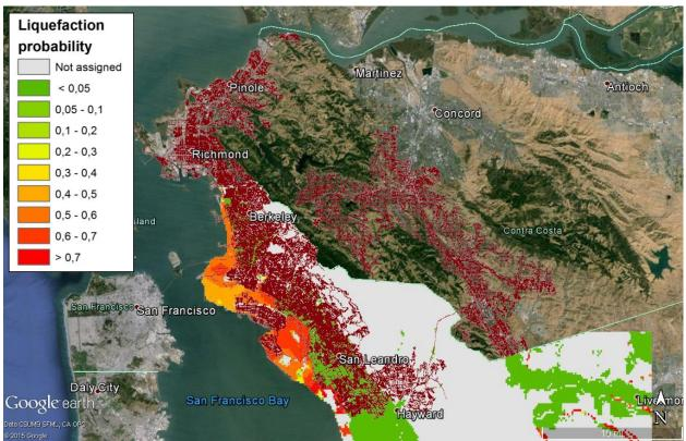
Figure 31. EBMUD water supply system with mainshock liquefaction probability
