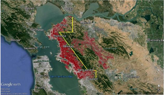
Figure 29. EBMUD system map (red) with dividing line (yellow) to approximately separate pipe and services east and west of the East Bay Hills
