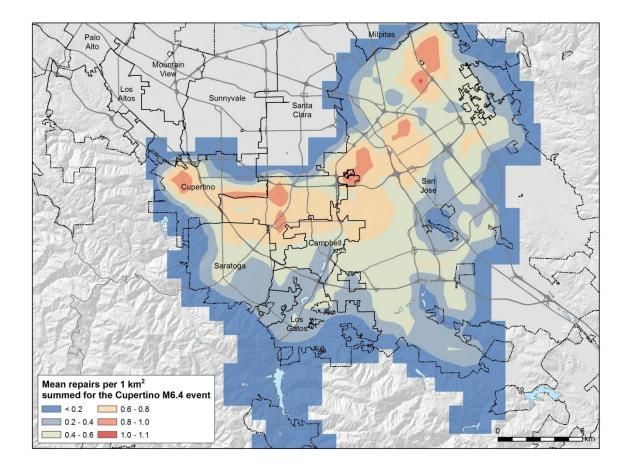
Figure 20. Buried water pipeline damage heatmap for Cupertino M 6.4 aftershock in SJWC's service area
