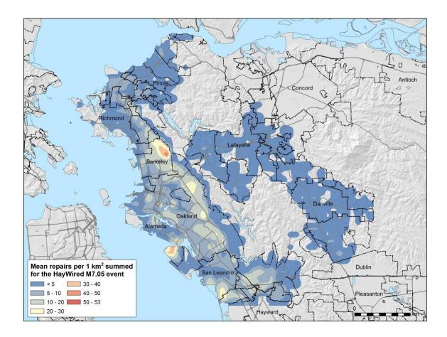
Figure 35. Buried water pipeline damage heatmap for the Hayward Fault mainshock in EBMUD's service area
