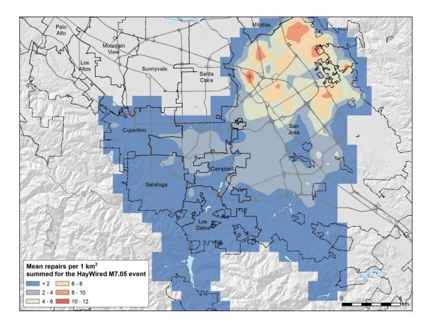
Figure 19. Buried water pipeline damage heatmap for the Hayward Fault mainshock in SJWC's service area
