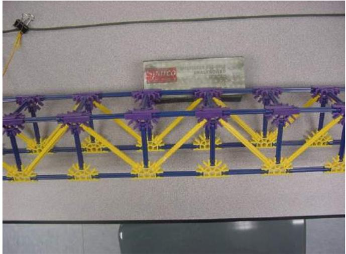
Run the cord (that's the main cable) though some eyelets or hooks in the ceiling and tie off the ends. Stack a couple desks (temporary shoring) on each other to get the deck near its final position. Run the string (that's the hangers connecting the main cable and the deck) through the deck and clip to the main cables (cords). Some raising and adjustment will be necessary – but the student reaction makes it well worth it.
