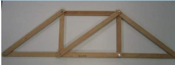
**Engineering Principle:** The basic equations required for analysis are the equations of equilibrium and trigonometry. However, no real numerical analysis is required. The model is used primarily for developing a feel for the basic definition for a truss: a structure composed of slender members joined together at end points by frictionless pins; loads only applied at joints; all truss members are 2-force members; and member weight is negligible.
