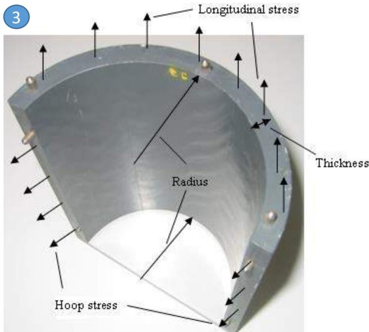
Using the model, help the students visualize how the internal pressure acts on the cylinder and generates internal stresses in the cylinder walls. Pull from the students that there are both internal stresses acting in the longitudinal and circumferential directions.
