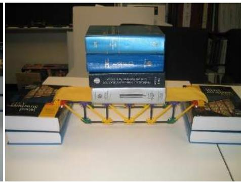
Weight the bridge, then the textbooks. There should be quite a significant difference in ratio between the weights. A light truss structure can support a load that is many times greater than the weight of the actual structural members over long spans.
