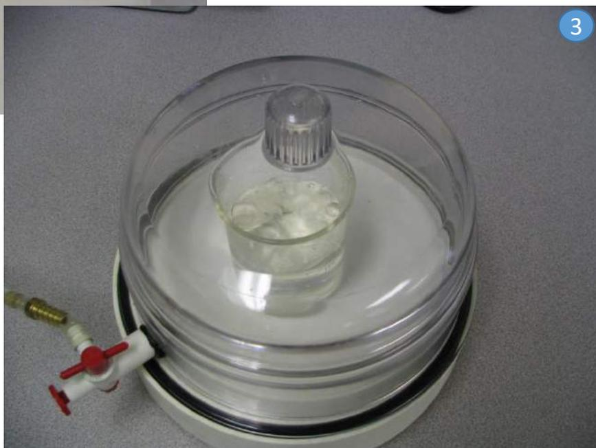
**Observations:** Students should be able to see vapor bubbles forming in the water in the beaker and then the water come to a rolling boil as the vacuum pump is turned on and evacuates the air from the pressure chamber. 3
