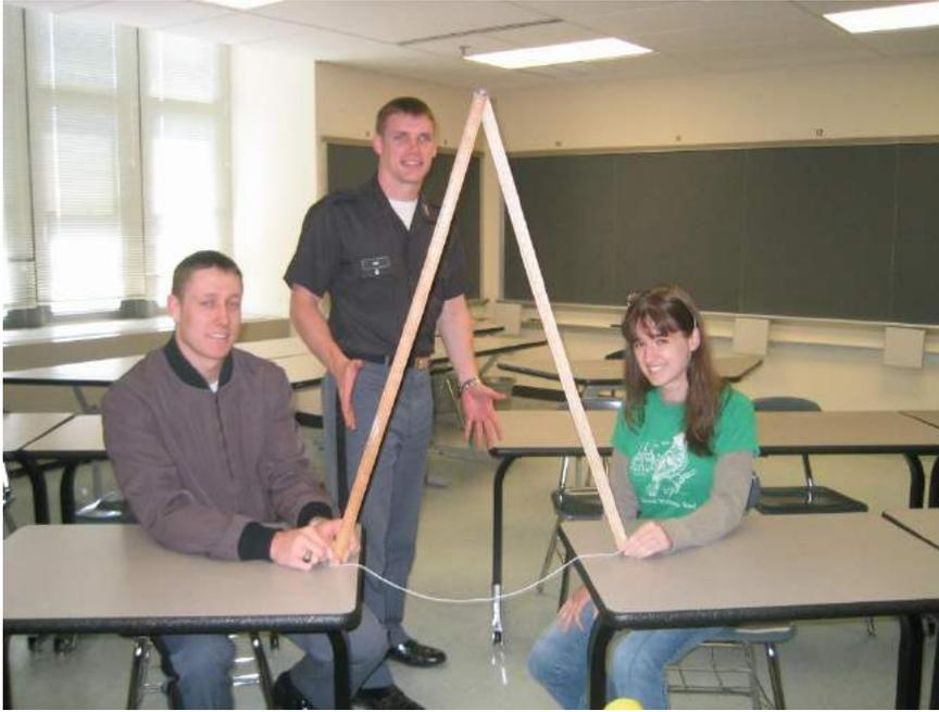
Ask another student to apply a force to the top of the rulers. The students holding the bottom using only their fingers should not be able to resist the outward movement of the rulers as the student presses down. Based on the loading applied, ask the students what type of load is in each leg of their simple truss? Pull from the students that the rulers are in compression while the string is in tension.
