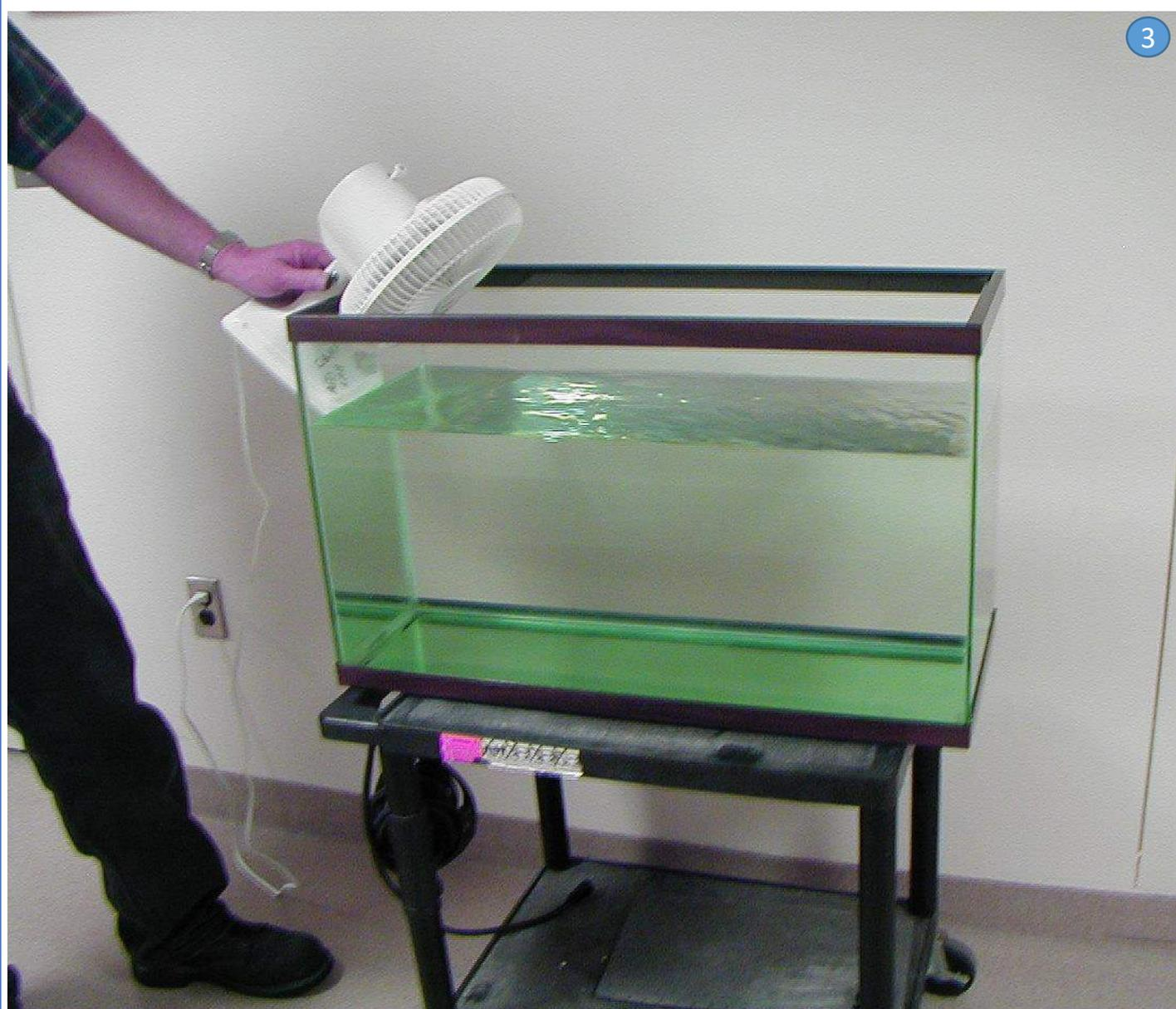
**Additional Application:** The deformation of the water surface can also lead into a discussion of viscosity as a measure of resistance to deformation (i.e. “What would happen if I replaced the water with honey and turned on the fan?”)
