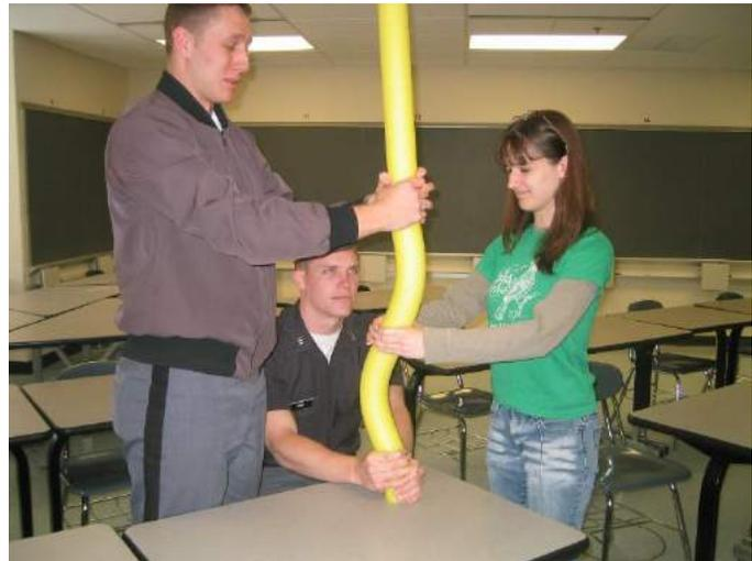
With vertical lines drawn along the length and horizontal lines drawn circumferential, torsional behavior can be displayed using the wacky fun noodle. A circular shape when twisted is experiencing pure shear and the squares created by drawing lines on the surface do not change size (area), but change shape (square becomes a rhombus – see rubber shapes physical models).
