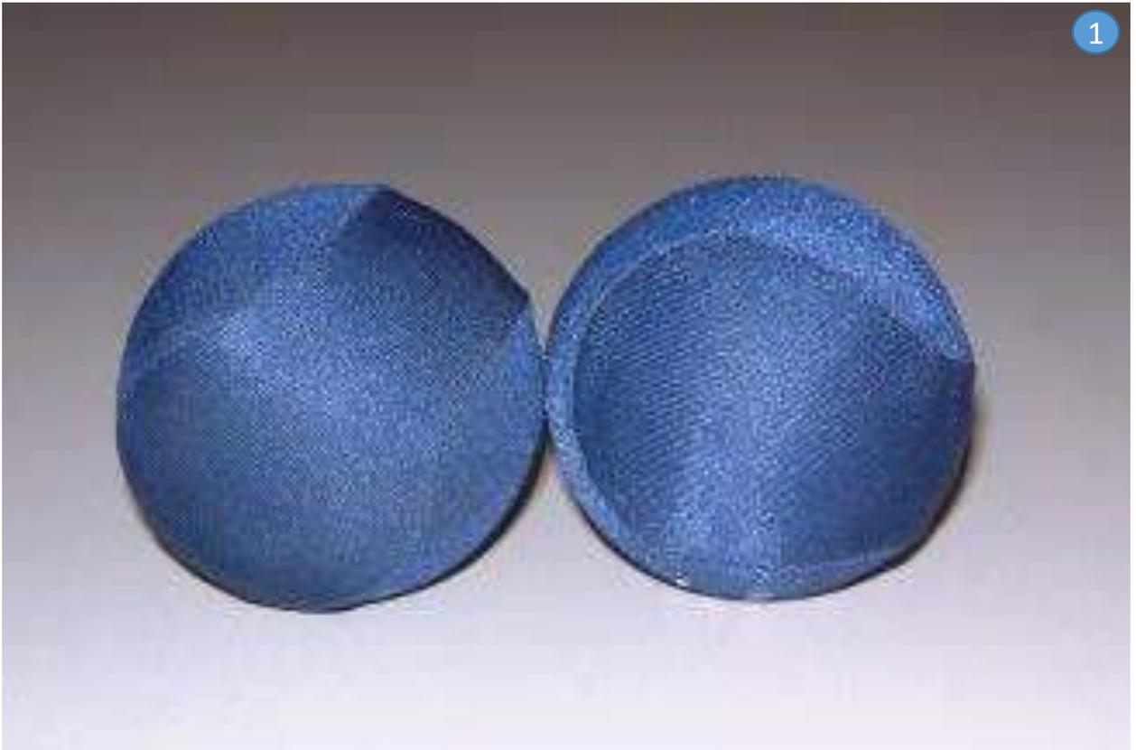
**Engineering Principle:** Two objects in a head-on or rear-end collision (“central impact”) will deform as they collide. At the time of maximum deformation, they will have reached the same velocity. The period of deformation will typically be followed by a period of restitution, at the end of which the two objects will either have regained their original shapes or will have retained some degree of permanent deformation.
