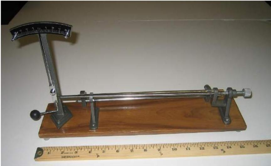
**Engineering Principle:** When materials, especially metals, are exposed to heat, they expand at different rates. The reverse is also true in that cold temperatures tend to cause material contraction. The amount of expansion/contraction may be small, but if not taken into account in the design of structures and/or machine parts, the resulting expansion/contraction could result in excessive strain/stress.
