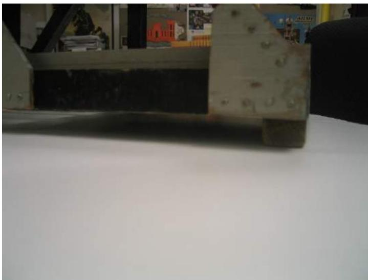
**Additional Application:** Using a sturdy wooden structure as described above, real issues such as overhead clearance, lateral supports, abutments, etc. can be discussed. Real looking connections that do not represent idealized pin connections are brought to life.
