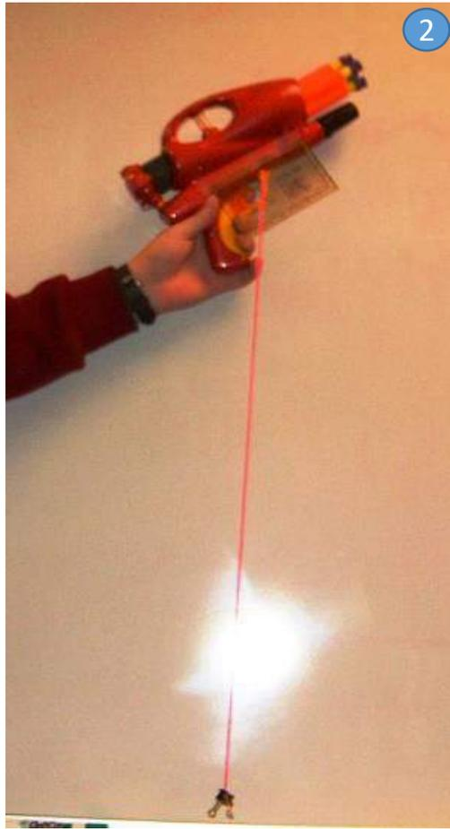
**In Class:** Introduce the equations above and use the toy gun to validate them. Use students as time keeper, recorder, impact point marker, etc.
