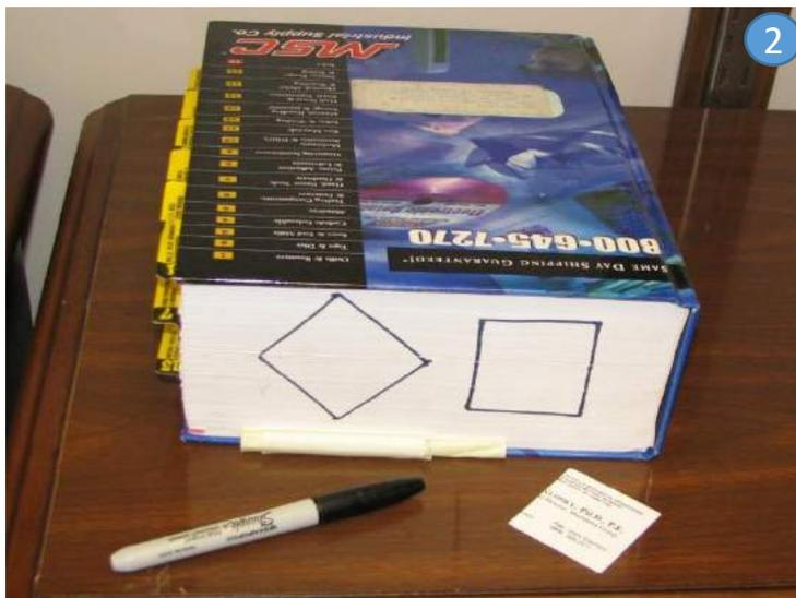
**In Class:** Point out to the students that the marks on the pages are the same size, and the only change is the orientation of the marks. Discuss the state of pure shear in detail, and then point out the fact that one of the blocks is in pure shear and one has no shear, even though they are drawn on the same pages. Draw Mohr's circle for the case of pure shear, with the circle centered at the origin, to illustrate how normal stresses still exist, and where they should expect to find them.
