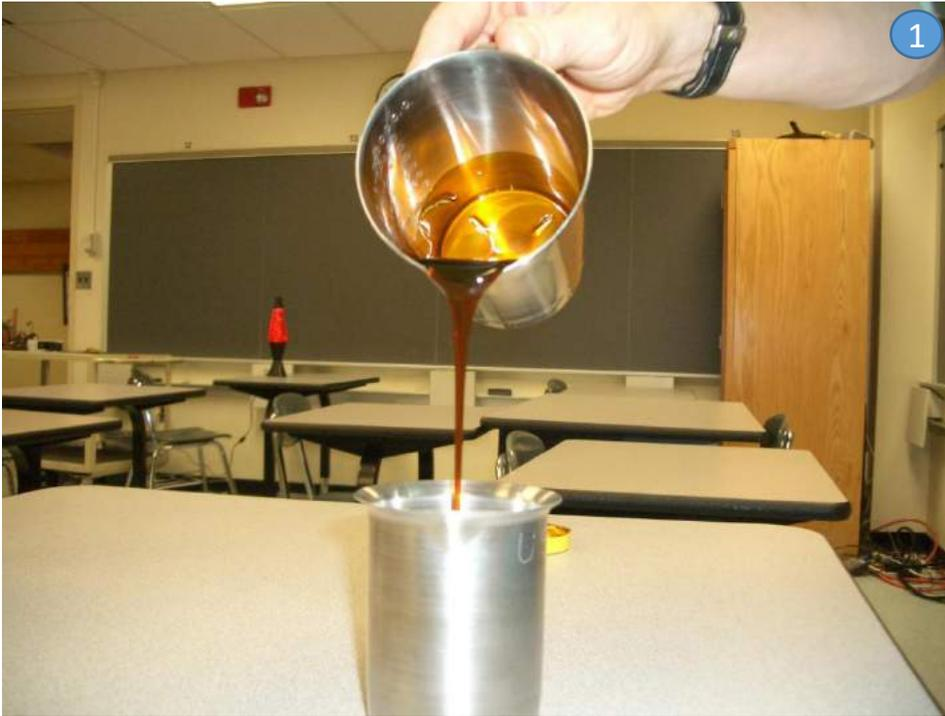
**Engineering Principle:** Mass is conserved when the mass flow rate into the system equals the mass flow rate out of the system:
