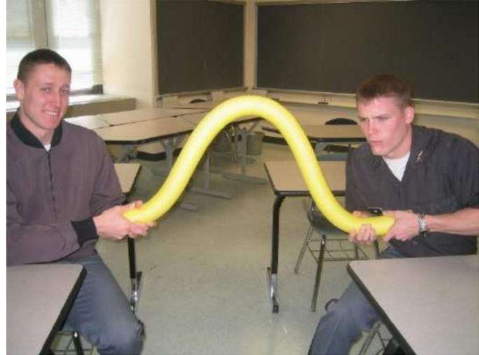
Ask the class what would happen if the length of the noodle where the force is being applied is decreased. Demonstrate, by asking the students to sit closer together as they apply force to the noodle (length decreased), that the effects of tension do not change but the compressive force needed to make it buckle is much greater.
