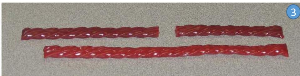
**Observations:** Point out the difference between deformation/strain in the elastic region (the Twizzler returns to its original length every time) and plastic region (permanent deformation).
