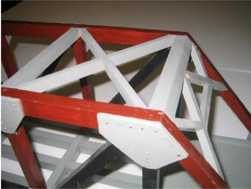
Partial abutments on either end: The bridge is built with a partial abutment on each end for placement on the two edges of the space being crossed. Abutments are necessary for real bridges and transfer the load from the bridge into the soil.
