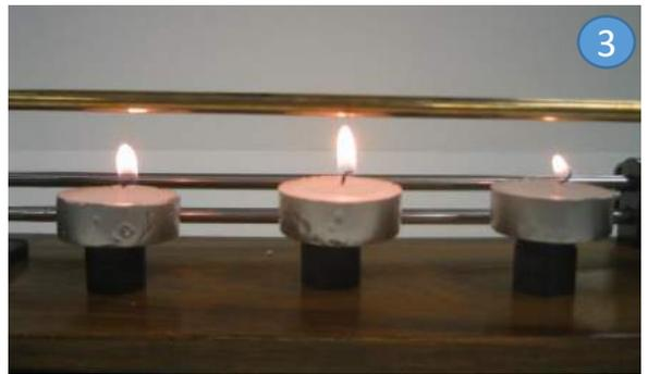
In any order, heat up each of the rods for about 10 minutes and make a note of how much the length of each changed. This experiment can be occurring while you are presenting the theory associated with thermal expansion. The students should see the brass expanding the most, then the aluminum, and the steel expands least.
