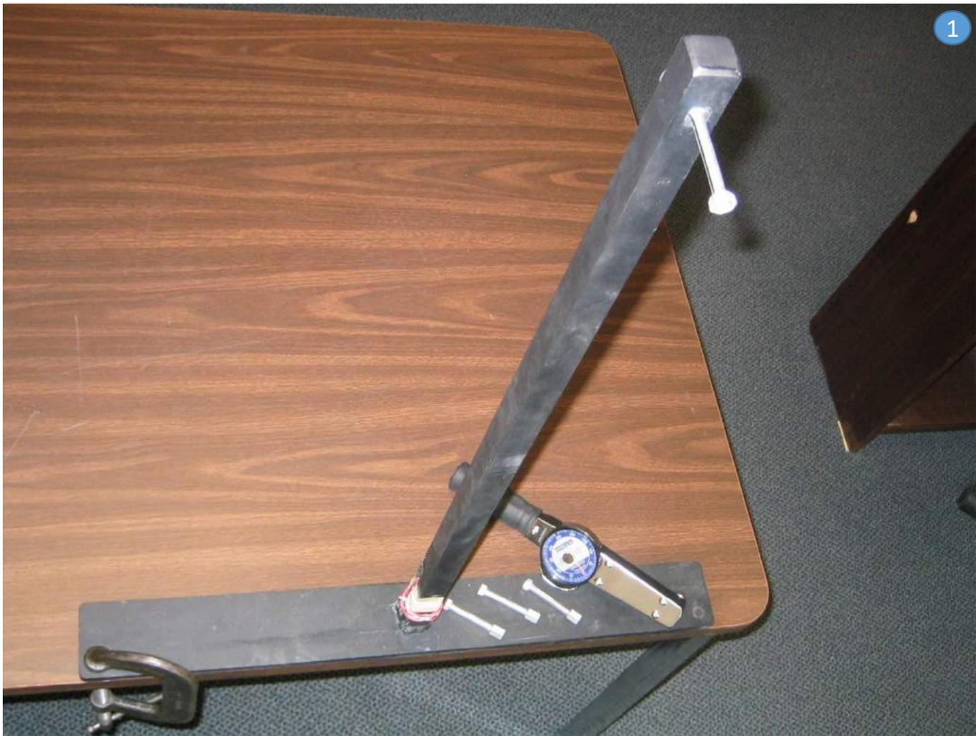
**Engineering Principle:** For cylindrical rods in torsion, the maximum shear stress experienced is seen at the outer surface, and for materials in the elastic range the shear stress is computed using the expression
