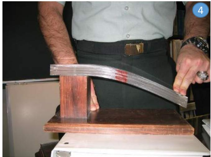
Show the students the demonstrator with the plastic strips attached to the base (cantilever). Ask what they think will happen to the beam and the square in the middle when you apply a force to the free side of the cantilevered beam. Press down on the beam and show how the square deforms (as the pieces of plastic slide). ④ Relate this to the shape of the square on the side of a cylindrical rod.
