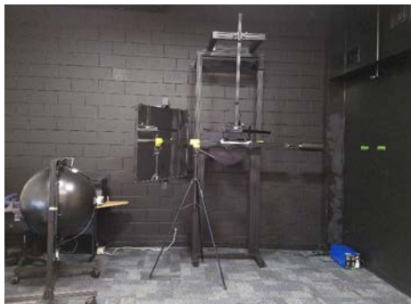
Figure 3: Wall-mounted goniophotometer (left); blackout shades and curtain-hanging system (right)
