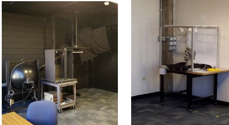
Figure 6: Cart with illuminance meter along with integrating sphere (left); frame with accent luminaires (right)
