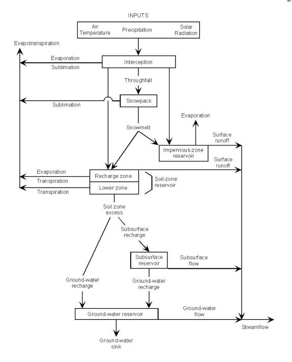
Figure 3.1. Schematic diagram of the conceptual system used in PRMS
