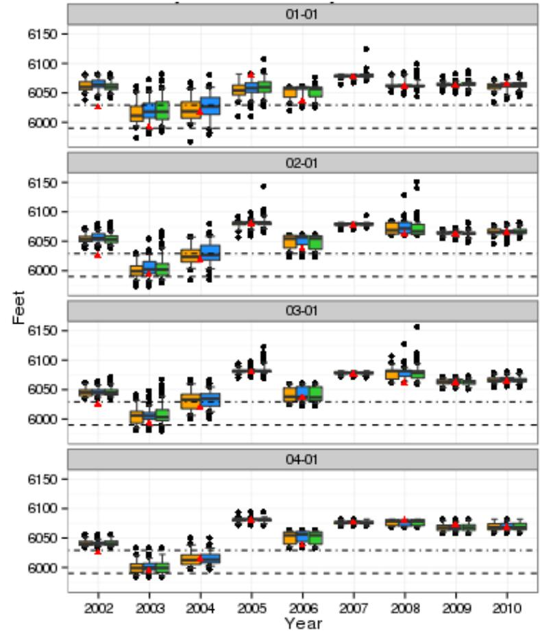
a) Computed Available Water: The dashed line is the 114,000 acre-foot threshold that if exceeded will allow for spring release from Navajo.
