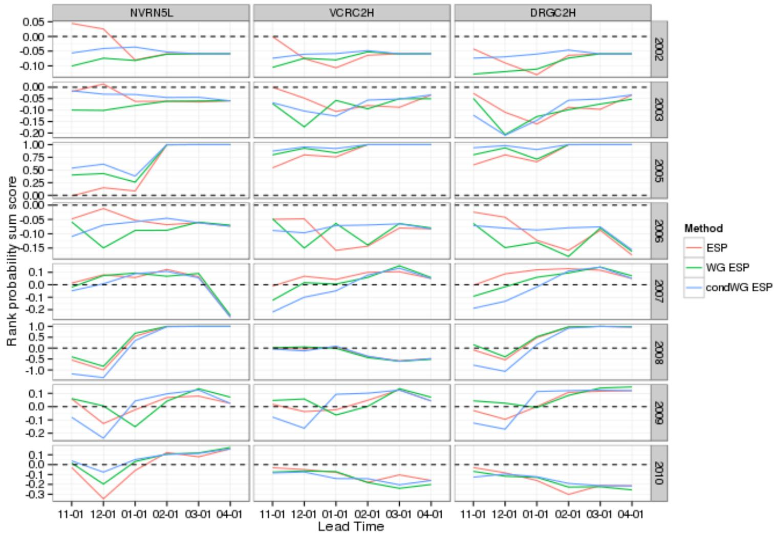
Figure B.7 RPSS values for each gage at each lead time for each year from 2002-2010. CondESP streamflow forecasting method performs better than the other methods for most of the years at early lead times.
