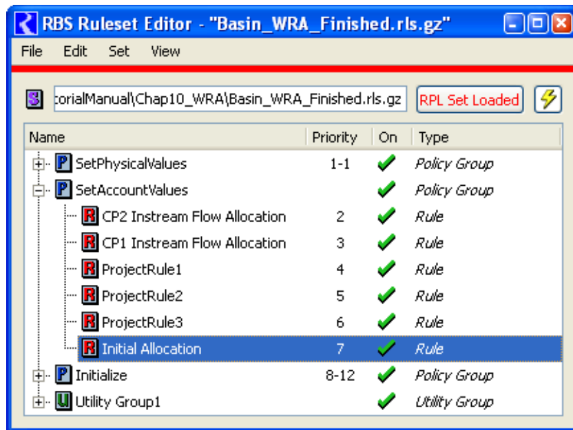
Figure 6. Example ruleset with initial allocation (rule 7), other operating rules (6, 5 and 4) and iterations of priority allocation for the instream flow (rules 3 and 2).
