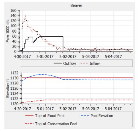
Figure 6. Plot of results from RiverWare after the first set of changes
