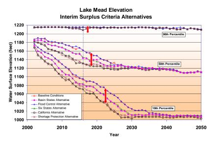
Figure 3. Application of the Graphical Policy Analysis Tool for comparing alternative operating policies on the Colorado River.
