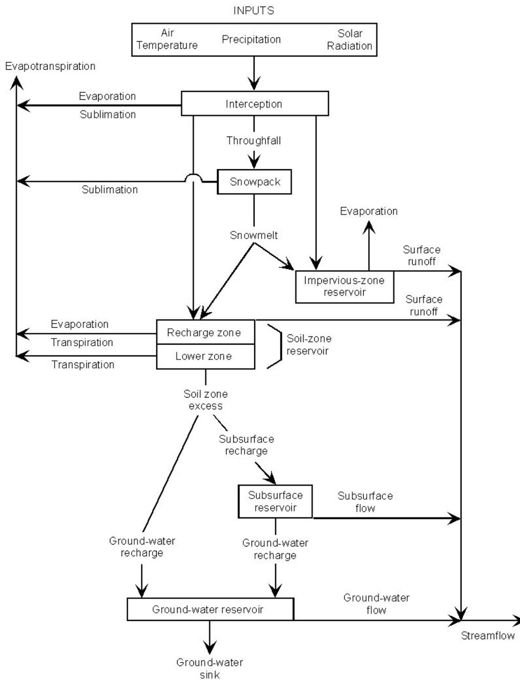
**Figure 3.1.** Schematic diagram of the conceptual system used in PRMS
