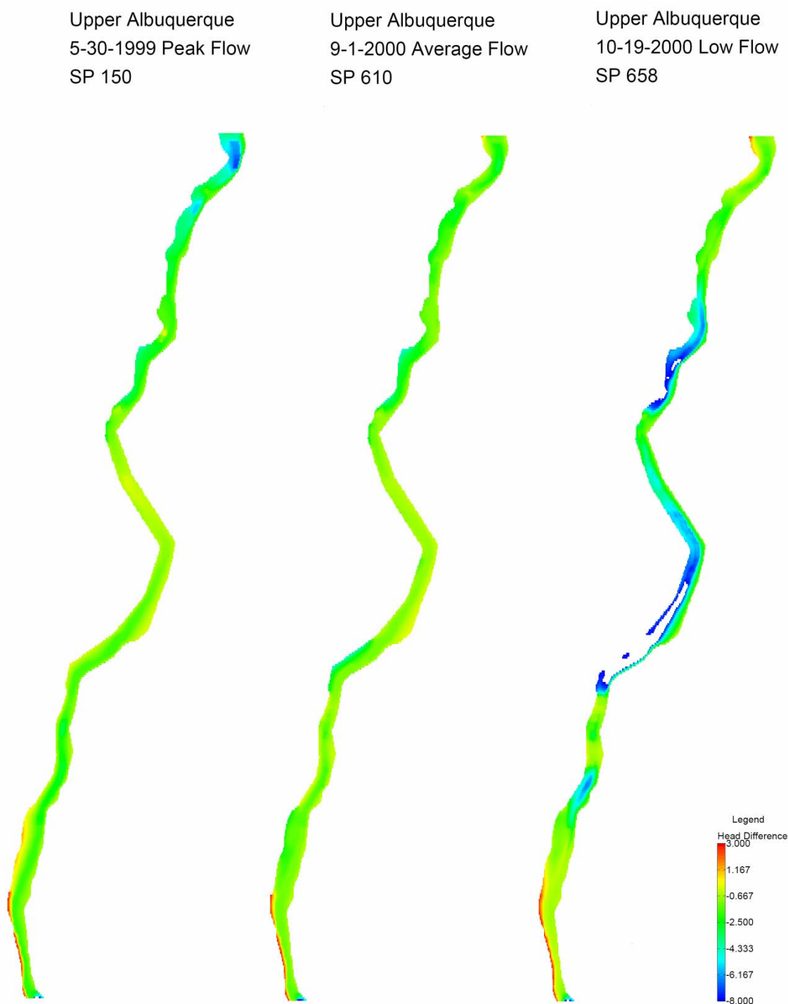
Figure 4.24a) Head Difference – Lower Portion of the Cochiti to Central Models 1999-2000 (UpperAlbuquerque). MODFLOW grid plan view is shown with color contours of the head difference between RW-MF Linked and MFOnly models (RW-MF Linked minus MFOnly). Color contours are shown for nominal dates in 1999-2000: peak flow event 5-30-1999, average flow event 9-1-2000, and low flow event 10-19-2000.
