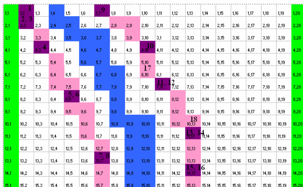
Figure 4.2) Test Model - MODFLOW Model Grid with Stream Segments Marked: RIV cells shown in blue, GHB cells are shown in green, cells which are overlain by STR/SFR segments are shown in pink and purple. The large bold numbers denote the STR/SFR Segment Number.
