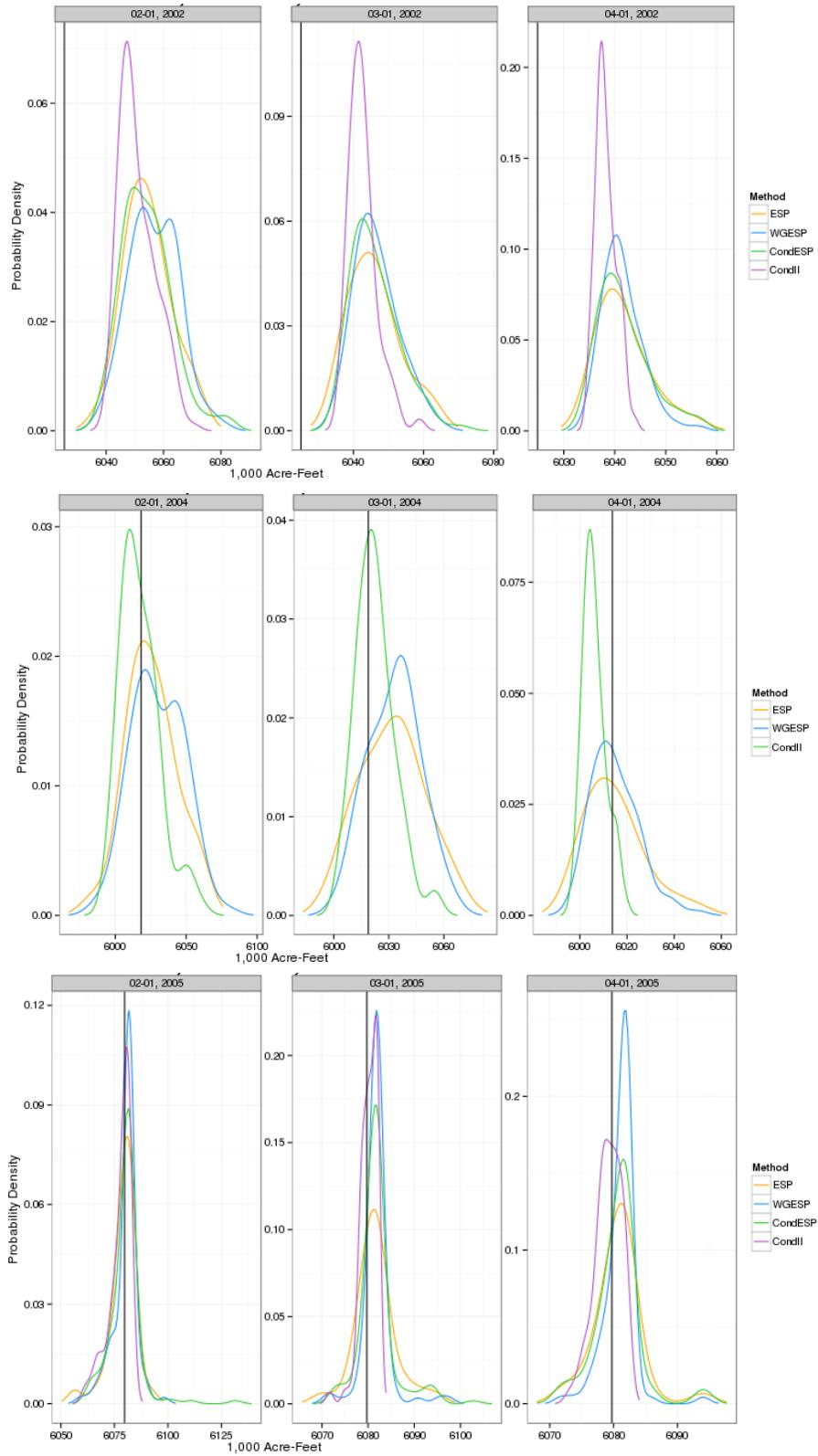
Figure 2.16 July pool elevation PDFs, top to bottom 2002, 2004, 2005.
