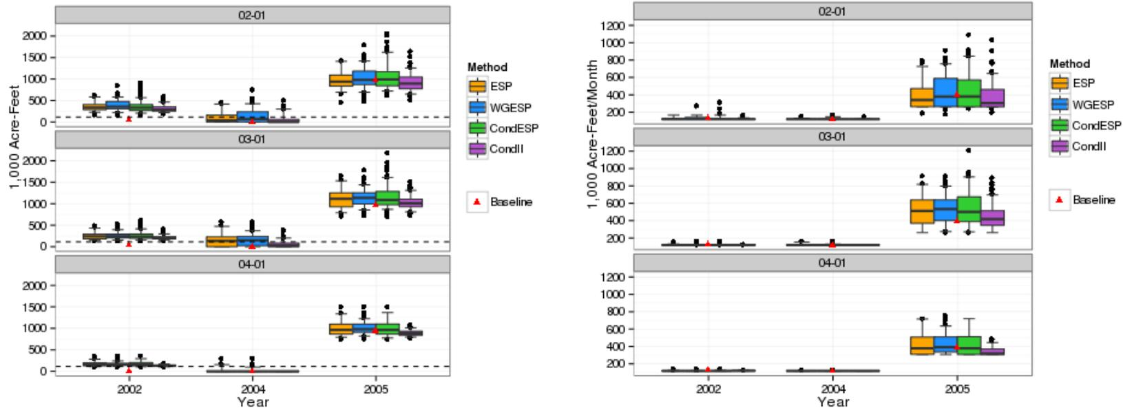
a) Computed Available Water: The dashed line is the 114,000 acre-feet threshold that if exceeded will allow for spring release from Navajo.
