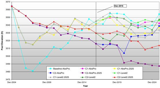
Figure 4-30 Powell 10<sup>th</sup> Percentile Elevation – C1 & C2 (2025)
