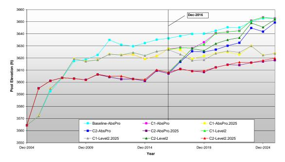
Figure 4-31 Powell 50<sup>th</sup> Percentile Elevation – C1 & C2 (2025)
