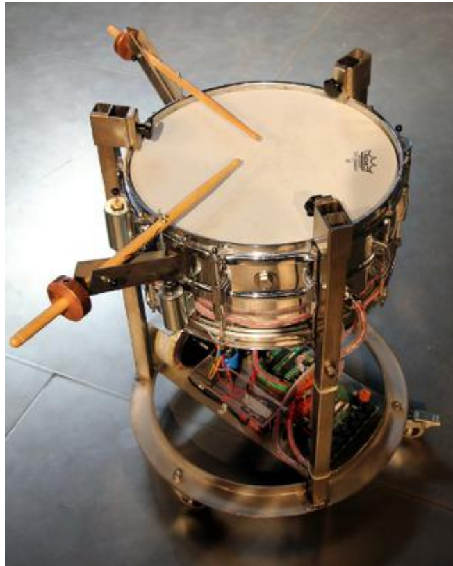
Figure 2.6 - Raes' <Snar_2>, built for Aphex Twin has two external drum sticks and many more internal to the drum
