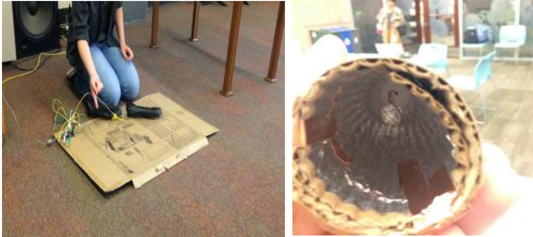
Figure 5.11 – More digital input designs: Interactive dance floor and tap shoes (left); a shake sensor made with a rock covered with aluminum foil (right)
