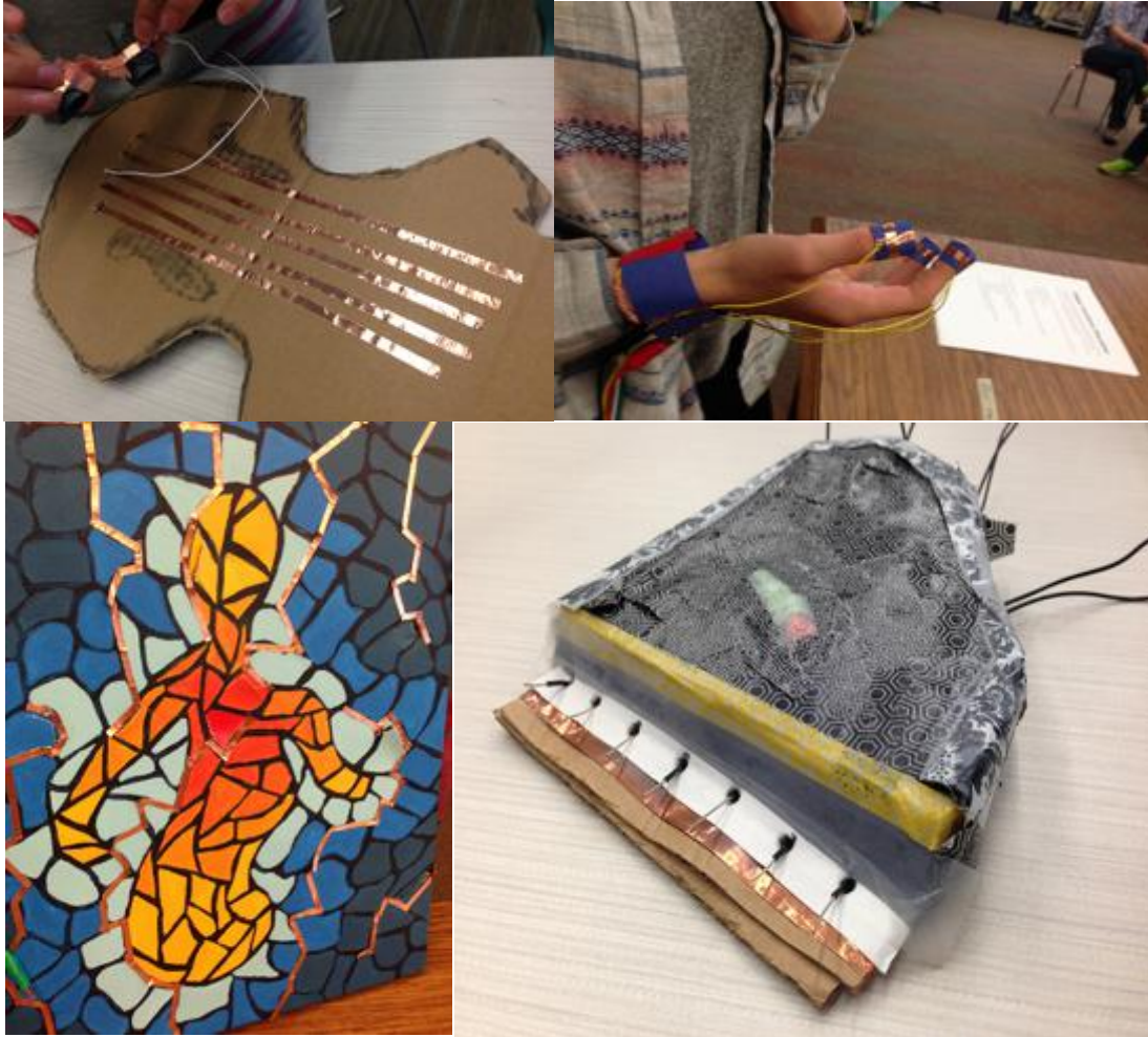
Figure 5.10 – Shielded wire supports movement, extending reach and other switch designs: A strumming interface; finger rings; interactive painting; mini-grand piano (clockwise from top left)
