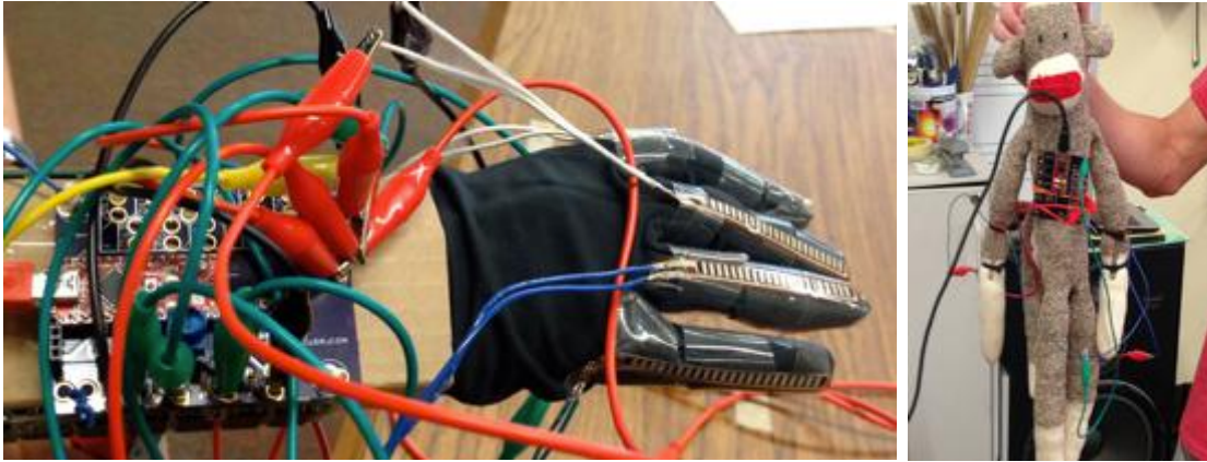
Figure 5.14 – Bend Sensors in different contexts: Glove based controller with bend sensors (left); Sock monkey stuffed animal with bend sensors in the arms (right)
