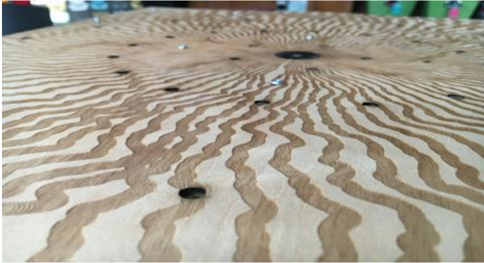
Figure 7.7 - Solarophone user interface with 42 light sensors
