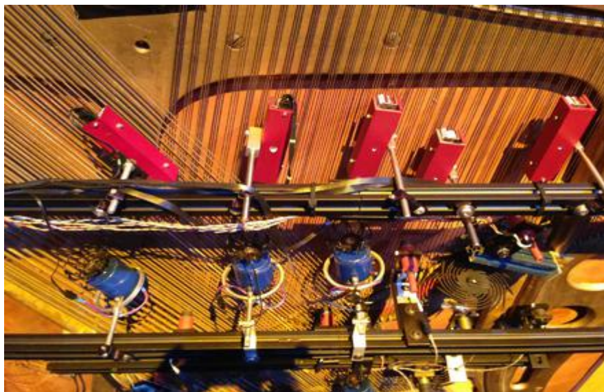
Figure 7.2 - Trimpin's 80/20 mounting system: shown on a piano harp installed for the 2015 ATLAS performance
