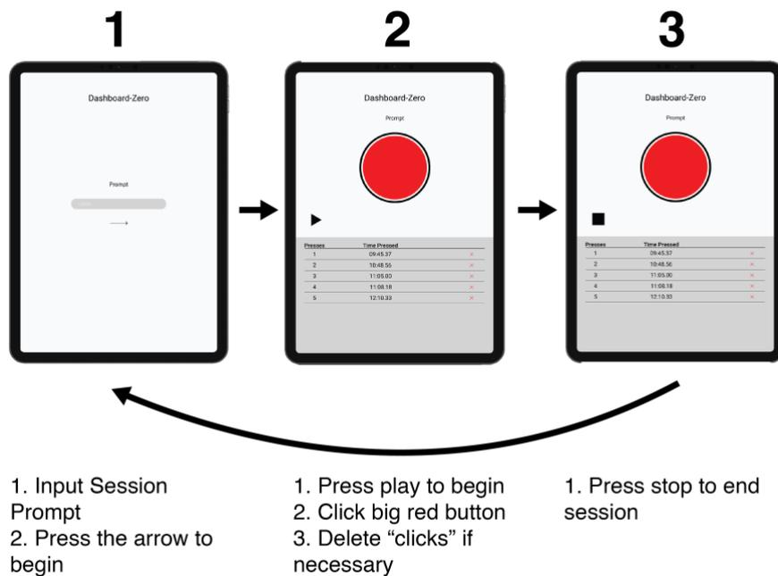
**Fig. 1.** The design of Dashboard-Zero was done in Figma, with the intent of passing on to a development team to incorporate into their research software. Above is the interface as seen by teachers while using it. This was intentionally designed as a very simple and customizable dashboard, so that research teams can adjust it to their needs
