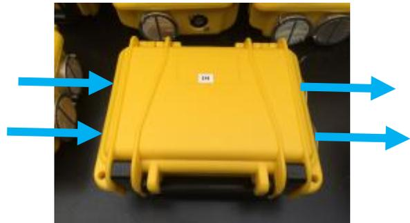
When the monitor is sealed the fan is pulling the sample in the left side inlet vents and out the vents on the right side of the pod. The fans inside of the pod (on the right side) pull air through the pod from the inlet through the outlet.
