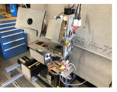
From big: this "beam mapper" allows us to measure a lens by moving a source along a hemispherical surface. We can move along (X,Y,Z) and Az+El angles, as well as polarization. Undergraduates have been involved in:
