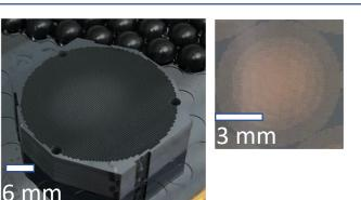
To small: Developing metamaterial lenslets which control light with sub-wavelength (micron-scale) features to make lenses which are superior to current hemispherical lenses.
