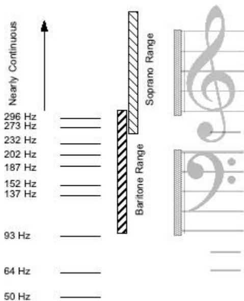
Figure 7. The strong resonances on the left hand side identified in Figure 6 are shown in relation to the approximate range of adult male and female voices and in relation to contemporary musical notation.
