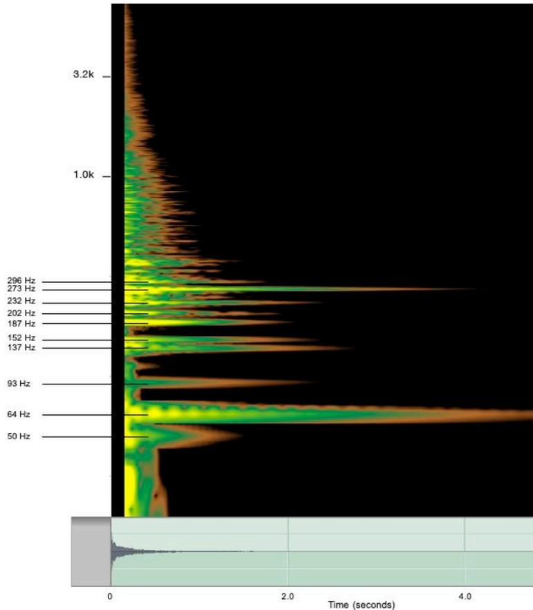
Figure 6. A sonogram of a recording of a balloon burst inside the temazcal and the six seconds thereafter. Note the modulation of the 64 Hz resonance first recognized by Thomason.
