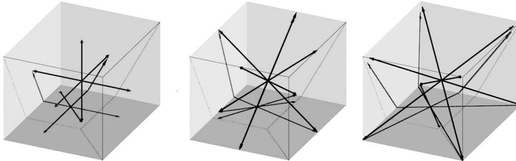
Figure 4. Room modes of a parallelepiped: planar, dihedral and trihedral.
