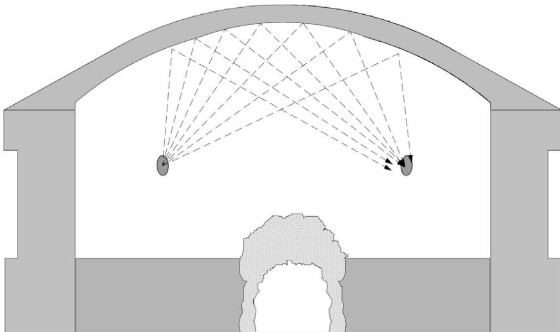
Figure 5. Ray tracing study illustrating effects of concave underside of the dome.
